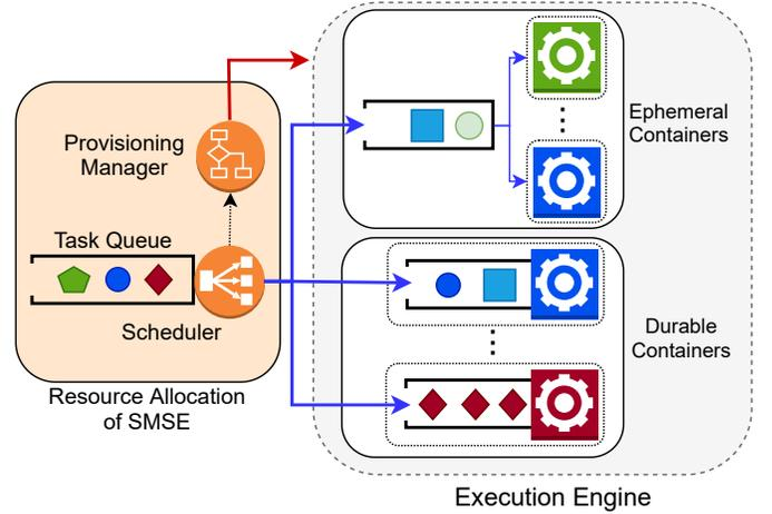
Fig. 4: An example of the Provisioning Manager module controlling function containers in two configurations. The top one has a centralized machine queue and creates one ephemeral container for each task. The bottom configuration shows in-memory durable containers for different functions (task types) where each container has a dedicated local queue that is accessible to the task Scheduler.
