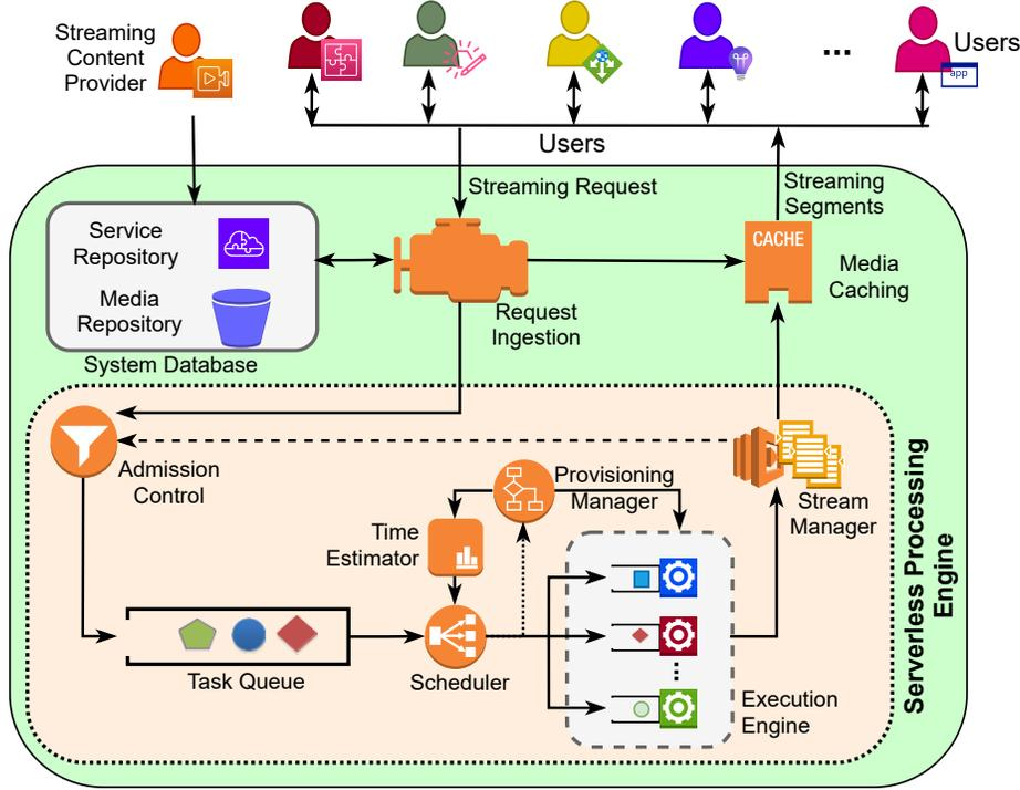
Fig. 2: Architectural view of the Interactive Serverless Media Streaming Engine (SMSE). The engine deals with the requests of stream providers and end-users. The service providers procure the content and functions to be applied on them. End-users can apply the defined services/functions while streaming the contents.
