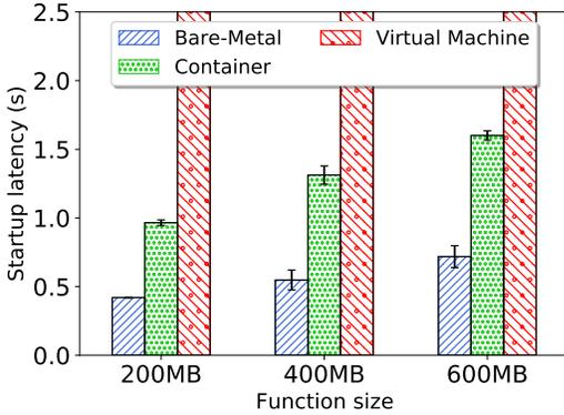
Fig. 5: Comparing the startup latency (overhead) of three Task Execution Unit deployments, namely bare-metal, container, and Virtual Machine (VM). The horizontal axis shows the size of the function and the vertical axis shows the time (in seconds) to launch the Execution Units.
