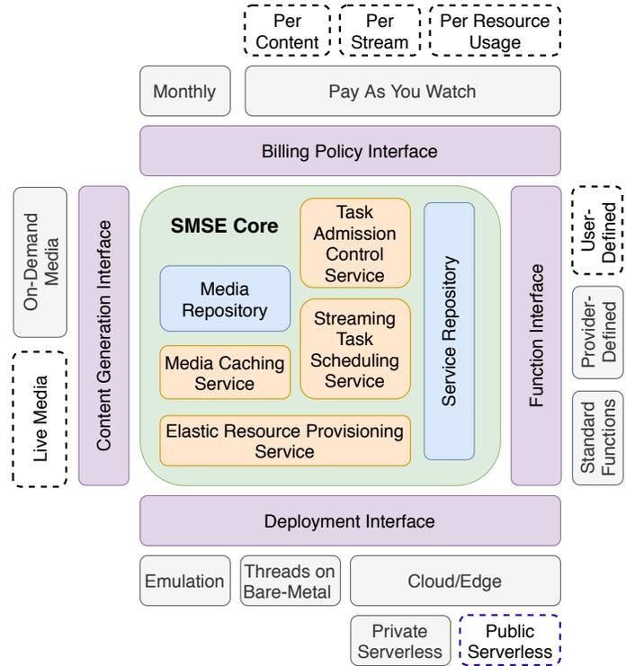
Fig. 3: Expandable Interfaces in Serverless Media Stream Processing Engine (SMSE). Purple boxes outside of the SMSE Core represent different interfaces that collectively make the system flexible. Dashed-line boxes indicate planned components that yet to be developed in the prototype.
