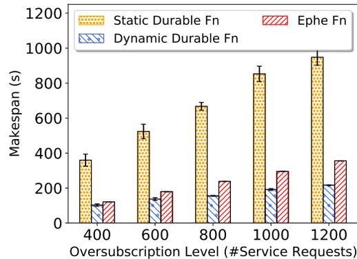
Fig. 7: Comparing the makespan time of completing different number of tasks arriving to SMSE within a fixed time interval (known as oversubscription level) using three different provisioning methods (static durable containers, dynamic durable containers, and ephemeral containers).
