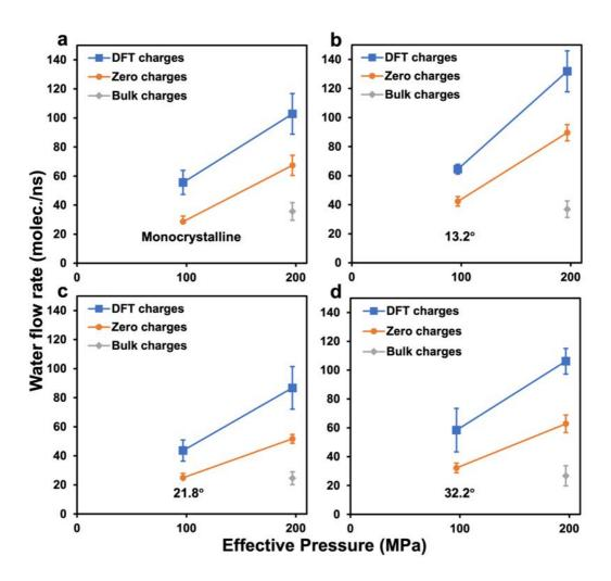
**Figure 11.** Water flow rate versus effective pressure plots for various configurations: (a) monocrystalline, (b) 13.2°-misoriented bicrystalline, (c) 21.8°-misoriented bicrystalline, and (d) 32.2°-misoriented bicrystalline nanoporous hBN membranes.
