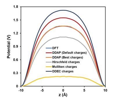
**Figure S8.** Electrostatic potential calculated using DDAP partial charges with default and customized parameters, Hirshfeld partial charges, Mulliken partial charges, DDEC partial charges, and direct DFT calculation for a monocrystalline nanoporous hBN membrane.
