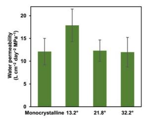
Figure 9. Water permeability at 46.87 MPa effective pressure for monocrystalline and bicrystalline hBN membranes.
