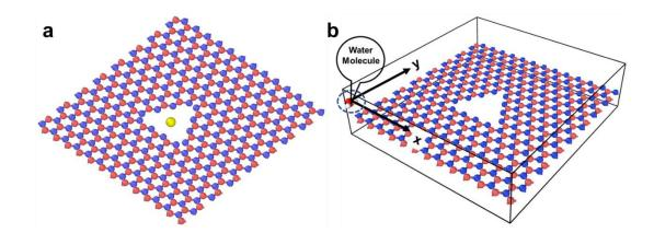
**Figure S3.** Snapshot of a nanoporous hBN membrane (boron in red and nitrogen in blue) depicting (a) a test charge atom (in yellow) at the centre of the nanopore and (b) a tangential water molecule at the corner of the membrane at a distance of 3 Å above the surface of the hBN layer.
