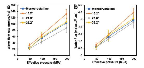
**Figure 8.** (a) Water flow rate and (b) water flux versus effective pressure for nanoporous monocrystalline and bicrystalline hBN membranes.
