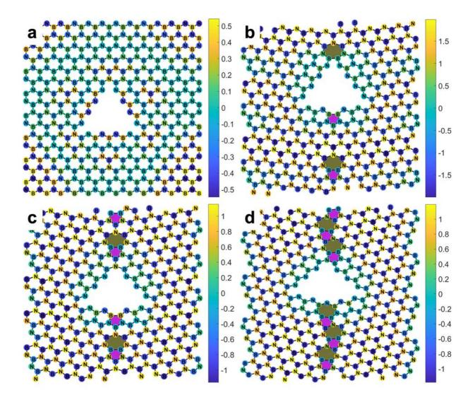
**Figure 4.** Partial charge (in elementary charge unit (*e*)) distribution calculated using the "best" DDAP parameters for various configurations: (a) Monocrystalline (b)  $13.2^{\circ}$ -misoriented bicrystalline, (c)  $21.8^{\circ}$ -misoriented bicrystalline, and (d)  $32.2^{\circ}$ -misoriented bicrystalline nanoporous hBN membranes, respectively. Five membered rings are colored in magenta and seven membered rings are colored in green.
