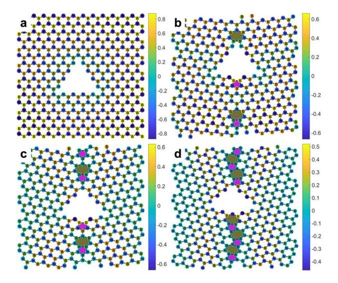
**Figure 3.** Partial charge (in elementary charge unit (*e*)) distribution calculated using the default DDAP parameters for various configurations: (a) Monocrystalline (b)  $13.2^{\circ}$ -misoriented bicrystalline, (c)  $21.8^{\circ}$ -misoriented bicrystalline, and (d)  $32.2^{\circ}$ -misoriented bicrystalline nanoporous hBN membranes, respectively. Five membered rings are colored in magenta and seven membered rings are colored in green.
