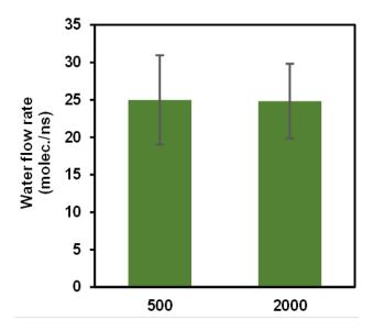
**Figure S1.** Water flow rate for nanoporous monocrystalline hBN membrane at 50 MPa feed pressure by considering 500 and 2000 water molecules on the permeate side.
