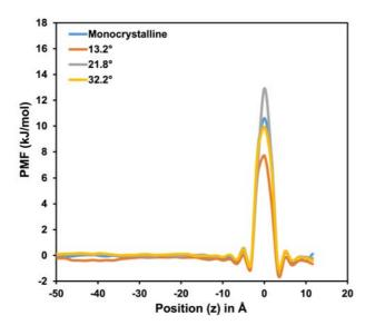
**Figure 10.** Free energy profile or PMF variations along the flow direction (*z*-direction) for nanoporous monocrystalline and bicrystalline hBN membranes of varying misorientation angles.
