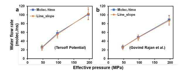
**Figure S7.** Water permeability versus effective pressure plots, calculated using two different methods, for a nanoporous monocrystalline hBN membrane when the membrane was simulated using: (a) the Tersoff force field<sup>20</sup> and (b) the force field developed by Govind Rajan et al.<sup>3</sup>
