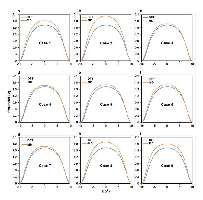
**Figure S6.** Electrostatic potential (in orange color) as a function of the out-of-plane distance from the centre of a 13.2°-misoriented bicrystalline hBN membrane for different sets of parameters using density derived atomic point charges: (a-i) cases 1 to 9 for different set of parameters, respectively. The DFT potential is shown in purple color in each case.
