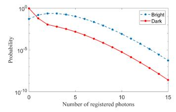
Figure 3. Identification of the state of a fluorescent qubit under conditions of significant registration errors. The following parameters were selected: t = 1,  $\lambda = 0.05$ ,  $\lambda_D = 0.05$ ,  $\lambda_B = 3$ .
