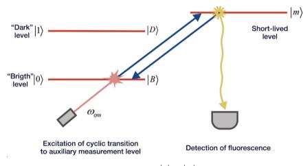
Figure 1. Excitation of a cyclic transition  $|0\rangle \rightarrow |m\rangle$  by resonant laser radiation.
