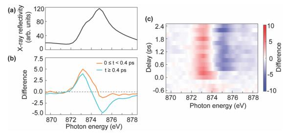
**Fig. 5** (a) The static X-ray reflectivity spectrum at the nickel L<sub>2</sub>-edge. (b) The difference spectra of the X-ray reflectivity with laser and without laser at transient time ( $0 \le t < 400$  fs, orange line) and at longer delays ( $t \ge 400$  fs, cyan line). (c) The map of the difference spectra as a function of delay and photon energy.
