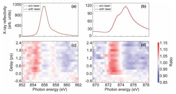
**Fig. 3** (a), (b) X-ray reflectivity spectra of NiO at the nickel  $L_{2,3}$ -edges. The dashed black and solid red lines represent the spectra acquired at time delays longer than 400 fs without and with laser excitation, respectively. (c), (d) The ratio map as a function of delay and photon energy at the nickel  $L_{2,3}$ -edges.
