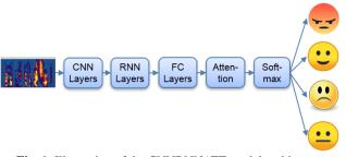
Fig. 1. Illustration of the CNNRNNATT model architecture
