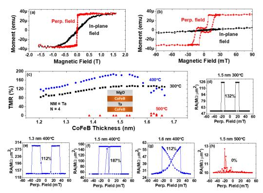
Figure 3. (a) Hysteresis loops of MgO/ CoFeB/Ta(1nm)/CoFeB/MgO measured on different magnetic fields. (b) The same curves at low field-region. (c) CoFeB thickness dependence of the TMR in pMTJs with Ta-MIFLs (Inset: schematic of Ta-MIFL). The samples were successive annealed at each temperature for 10 min. (d) TMR curve of the 1.5 nm sample after the 300°C annealing. (e-g) TMR curves of three pMTJs after the 400°C annealing. (h) TMR of the 1.5 nm sample after the 500°C annealing.
