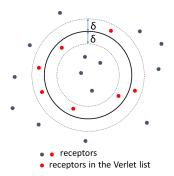
FIG. 4. The Verlet list employed for mobile ligand systems contains all receptors with distances from the edge of the disk smaller than  $\delta$ . A new list is initialised once the disk diffuses a distance bigger than  $\delta$ .
