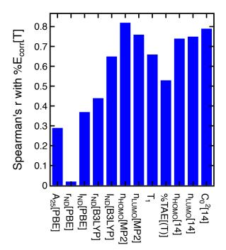
**Figure S7.** Bar plot of Spearman's *r* for  $\&E_{corr}[(T)]$  with different MR diagnostics on the 10,000 TMCs. Fourteen active orbitals are used for the CASSCF calculations
