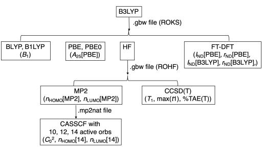
**Figure S16.** Workflow of computing 14 MR diagnostics. All calculations were performed with ORCA 4.0.2.1<sup>17-18</sup>.
