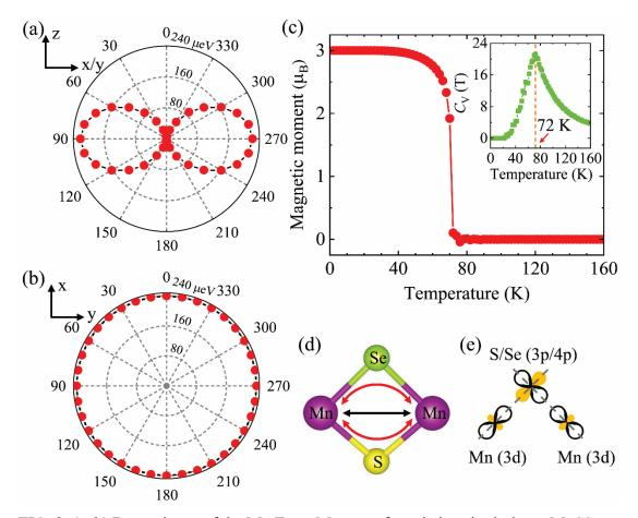
FIG. 3. (a, b) Dependence of the MAE per Mn atom for pristine single-layer MnSSe on the out-of-plane polar angle  $\theta$  and in-plane azimuth angle  $\varphi$ , respectively. (c) The simulated magnetic moment and specific heat ( $C_v$ ) with respect to temperature. (d) Schematic mechanism of direct Mn-Mn (black arrows) and super-exchange Mn-S(Se)-Mn (red arrows) interactions. (e) Mechanism of super-exchange interaction for a nearly 90° Mn-S(Se)-Mn bond angle.
