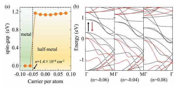
FIG. 5. (a) Variation of the band gap of spin-down channel with charge carrier concentration. (b) Three typical spin-polarized band structures.
