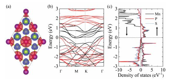
FIG. 2. (a) Spin-resolved charge density with an iso-value of 0.01 e/Å3 in the FM state. Red (blue) ones indicate the positive (negative) values. (b) Spin-resolved electronic band structures. The black (red) line represents the spin-up (spin-down) bands. (c) Projected density of state. In (b) and (c), the Fermi level is denoted by the dotted line at zero.
