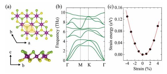
FIG. 1. (a) Top and side view of a MnSSe monolayer with 1T phase, where Mn, S, and Se atoms are purple, yellow, and green, respectively. The orange shaded region indicates the primitive unit cell. (b) Calculated phonon dispersion for 2D MnSSe crystal. (c) The strain energy of MnSSe monolayer under uniaxial strain.
