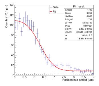
**Figure 15**. Fit result of the absorption points around the Gd grating edge. The blue histogram data is an excerpt of the data in Figure 14 for  $x_i$  modulo  $d_m > 5.0 \,\mu\text{m}$ . The red line shows the result of the least squares fit of Equation 3.6 to the data.
