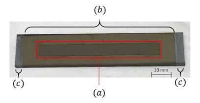
**Figure 3**. Detector used in the measurement of the spatial distribution of quantized UCNs. (a) - (c) indicate the following regions: (*a*) nuclear emulsion, (*b*) Si substrate and <sup>10</sup>B<sub>4</sub>C-NiC-C layer, (*c*) plain Si substrate.
