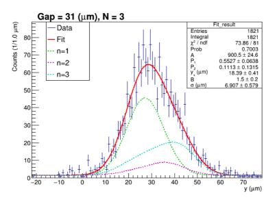
**Figure 19**. Fit result using Equation 4.11, which includes the effect of blurring. The effective gap was fixed to 31  $\mu$ m and the maximum number of the quantum state was 3. The blue histogram shows the distribution of obtained absorption points. The red line shows the best fit result obtained with model f(y). Dashed lines of green, purple, and light blue show the probability distributions of the ground state, the first excited state, and the second excited state, respectively.
