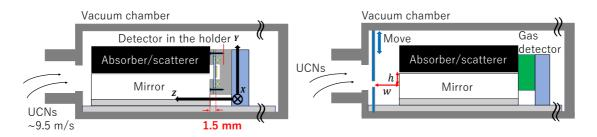
**Figure 16**. Setup for obtaining the quantized spatial distribution of UCNs. The figures on the left and right show the schematic view of the setup of the measurement of coordinates and velocity of UCNs, respectively. The distance from the exit of the mirror and absorber/scatterer to  ${}^{10}B_4C$  layer is 1.5 µm.
