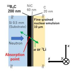
**Figure 1**. Schematic cross-sectional view of our high-resolution nuclear emulsion detector for cold neutrons and UCNs. Neutrons enter into the detector from the left. A  ${}^{10}B_4C$  layer converts the neutrons to  $\alpha$ -particles and  ${}^{7}Li$  particles, emitted back-to-back. Both of these create a track in the emulsion on the right side.
