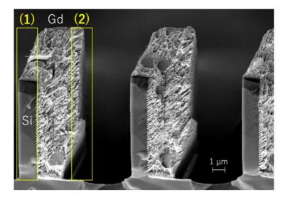
**Figure 8**. Electron micrograph showing a cross section of a Gd grating that was manufactured by the same process as that used in this experiment. The thickness of Gd in (1) is not sufficient to prevent cold neutrons from passing. We used the transmission image of the edge (2) for the estimation of the resolution of the detector.
