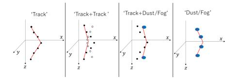
**Figure 9**. Classification of the reconstructed tracks. The reconstructed tracks were classified into four types. Red lines show reconstructed tracks. Black dots show silver particles. White dots of 'Track+Track' show silver particles on a track originally belonging to a different track than that of black dots. Blue ellipses of 'Track+Dust/Fog' or 'Dust/Fog' show fog or dust.
