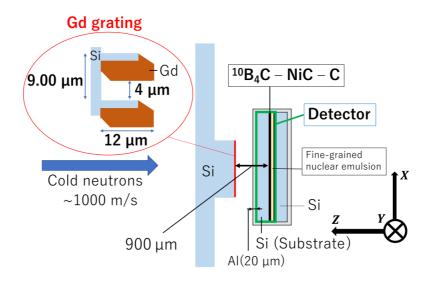
**Figure 7**. Setup for the measurement of cold neutron detection resolution. The Gd grating is located on the downstream side of a Si-slab placed in front of the detector. A Si plate was inserted to separate the emulsion layer from the Al foil to avoid the chemical effects of Al on the emulsion.
