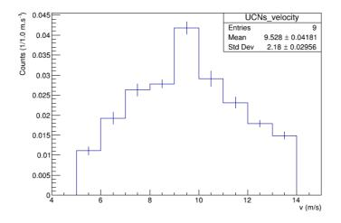
**Figure 17**. Measured velocity distribution at the UCN beam of the PF2 installation. The counts of UCNs of 4 - 11 m/s were measured using a gas detector with a <sup>10</sup>B layer.
