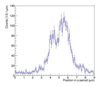
**Figure 14**. Distribution of  $x_i$  modulo  $d_m$  in the Gd transmission measurement. The resolution of the detector was evaluated using  $x_i$  modulo  $d_m > 5.0 \,\mu\text{m}$  whose region corresponded to the sharp edge of Gd grating.
