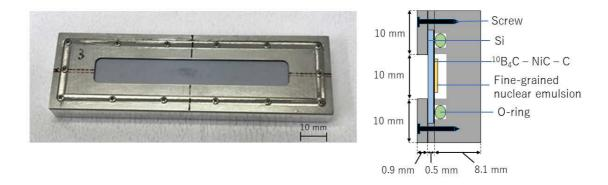
**Figure 6**. Holder allowing in-vacuum use of the emulsion detector. (left: photograph of the holder, right: schematic view of its cross section). The central part of the top cover of the holder was hollowed out to allow direct exposure of the surface of Si to vacuum. The yellow part of the schematic view shows the nuclear emulsion layer; the volume around it is kept at atmospheric pressure.
