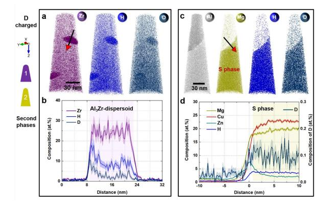
*Fig. 2. APT* analysis on second-phases of the D-charged AI-Zn-Mg-Cu samples in the peak-aged *condition* (120°C/24h). Atom map and composition profiles are presented along the red arrows respectively for (*a,b*) Al<sub>3</sub>Zr-dispersoids and (*c,d*) S-phase. The shaded regions in the profile corresponds to the standard deviations of the counting statistics in each bin of the profile; APT: atom probe tomography.
