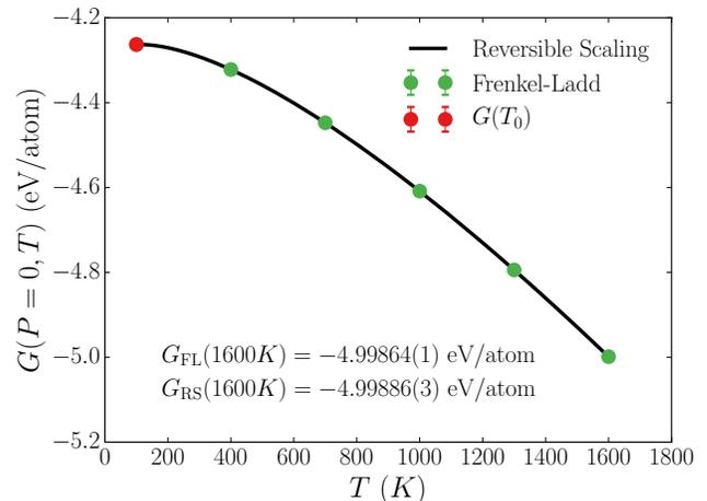
FIG. 3. Free energy per atom of the bcc phase of pure iron at zero pressure. The reference point for the RS path was at  $T_0 = 100$  K and  $P = 0$ . The FL calculations at other temperatures were used to verify the agreement against the RS result at high temperatures.
