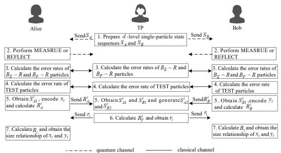
Fig. 1 The flow chart of the proposed SQPC protocol of size relationship
