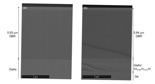
Fig. 6. Cross-section SEM images at  $30K \times$  magnifications of a (a) bulk GaAs-based DBR, (b) Ge-based DBR.
