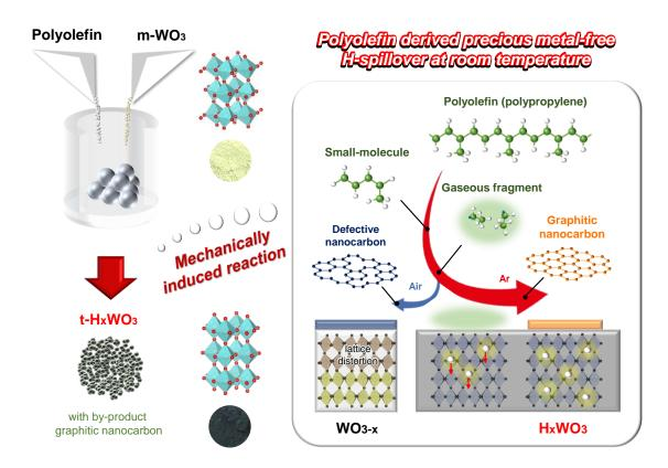
Fig. 9. Schematic illustration of the room-temperature synthesis of  $H_xWO_3$  in mechanically induced H-spillover.
