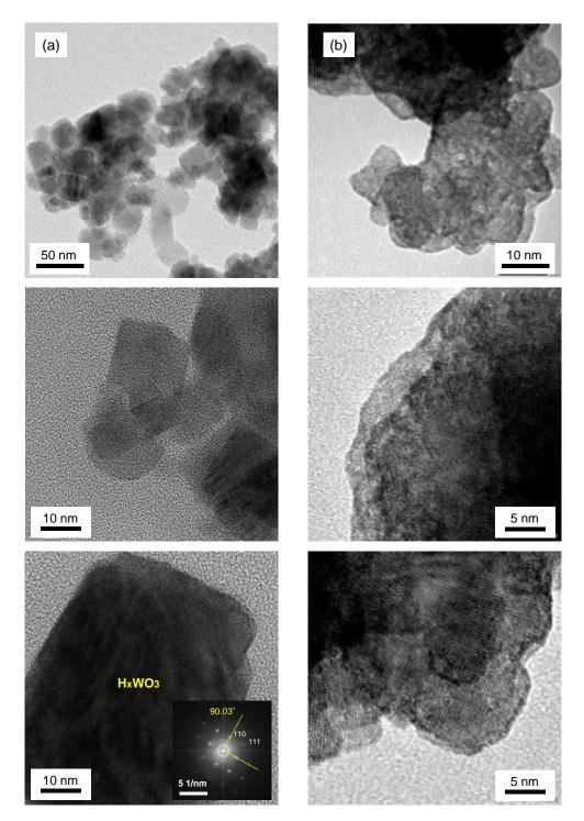
**Fig. 2.** TEM images; (a) the H<sub>x</sub>WO<sub>3</sub> nanoparticles (sample "S2", left side), (b) the ballmilled WO<sub>3</sub> nanoparticles without PP (sample "S1", right side).
