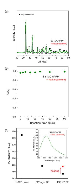
**Fig. 7.** Evaluation of the thermally treated sample; (a) XRD pattern, (b) the photocatalytic performance, and (c) comparison of PL intensity (the inset indicates PL spectra of S3).
