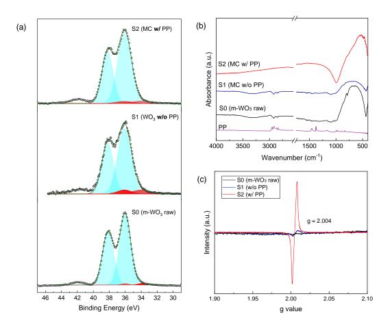
Fig. 4. (a) XPS spectra (W4f orbital), (b) FT-IR spectra, and (c) ESR spectra.
