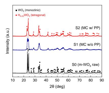
Fig. 1. XRD patterns of the raw and the pristine m-WO<sub>3</sub> powders after the ball milling.
