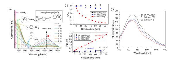
**Fig. 6.** (a) photocatalytic activity for the degradation of MO by S2 (synthesis with PP), (b) concentration change during visible-light irradiation (>385 nm), (f) photocatalytic reaction rate, and (c) PL spectra.
