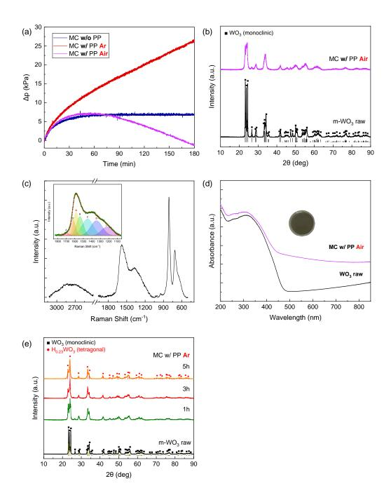
**Fig. 8.** Comparison of synthesis with the different atmospheres (Ar vs. Air); (a) in situ measurement of pressure change in the zirconia vessel during ball milling, (b) XRD patterns, (c) Raman spectra, (d) UV-vis spectra. (e) XRD patterns of prepared samples with varied treatment time.
