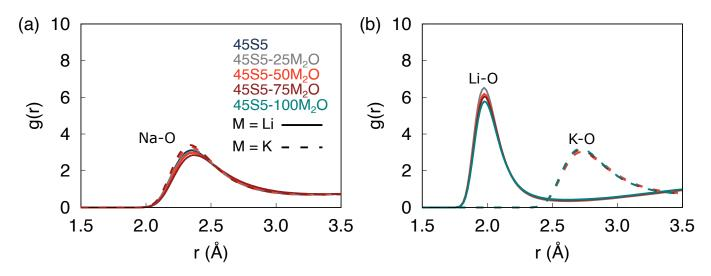
FIG. 9. (a) Na–O and (b) Li and K–O pair distribution functions in both Li mixed-alkali (solid lines) and K mixed-alkali (dashed lines) 45S5 bioactive glasses at 300 K.
