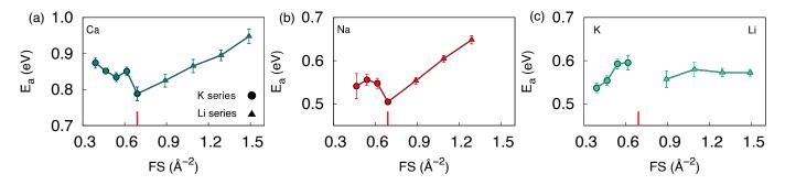
FIG. 5. The activation energies  $(E_a)$  of (a) Ca, (b) Na, and (c) Li or K as a function of the mean-field strength in the mixedalkali 45S5 bioactive glass. The  $E_a$  was calculated from the fitting of the lnD vs 1000/T with the Arrhenius function. Filled circles indicate data for potassium mixed-alkali 45S5, while filled triangles are for lithium mixed-alkali 45S5 bioactive glasses. The red vertical lines indicate the pristine 45S5 bioactive glass. The error is estimated from the fit.
