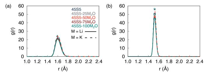
FIG. 7. Si–O (solid lines) and P–O (dashed lines) pair distribution functions in both (a) Li mixed-alkali and (b) K mixed-alkali 45S5 bioactive glasses at 300 K.
