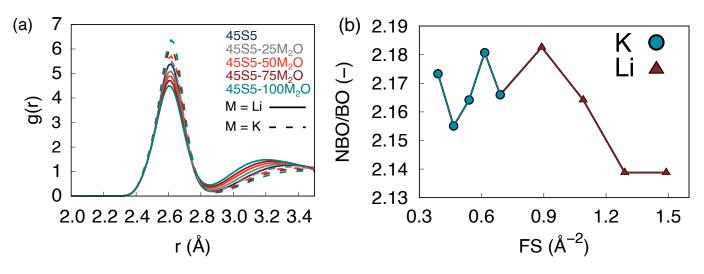
FIG. 10. (a) The O–O pair distribution functions in Li mixed-alkali (solid lines) and K mixed-alkali 45S5 (dashed lines) bioactive glasses at 300 K, (b) the NBO/BO ratio as a function of the mean field strength.
