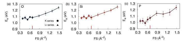
FIG. 4. The activation energies ( $E_a$ ) of (a) O, (b) Si, and (c) P as a function of the mean-field strength in the mixed-alkali 45S5 bioactive glass. The  $E_a$  was calculated from the fitting of the lnD vs 1000/T with the Arrhenius function. Filled circles indicate data for potassium mixed-alkali 45S5, while filled triangles are for lithium mixed-alkali 45S5 bioactive glasses. The red vertical lines indicate the pristine 45S5 bioactive glass. The error is estimated from the fit.
