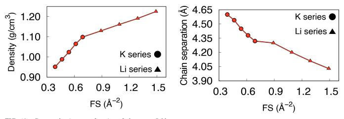
FIG. 13. Oxygen density as a function of the mean field strength at 300 K. Filled circles indicate data for potassium mixed-alkali 45S5, while filled triangles are for lithium mixed-alkali 45S5 bioactive glasses. The data is averaged over the last 100 ps from an NVT run, and the error bars are within the size of the symbol and are removed for clarity.
