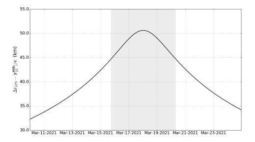
Figure 2. First-order 2-way relativistic time delay correction,  $\delta t_{1PN}$ , on the first BepiColombo superior solar conjunction. The peak value, occurring when the impact parameter is at its minimum, is 50.6 km. The gray shaded area indicates that b is below 7 solar radii.
