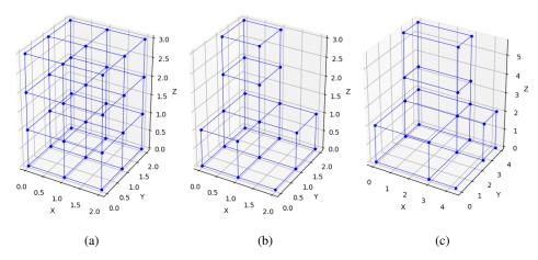
Figure 1: A frame structure is created from a regular 3D grid (a), removing cubes (b) and then changing the length of beams (c).
