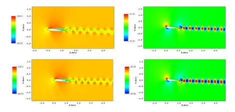
Fig. 6: Velocity along the x-axis (left) and y-axis (right): comparison between a simple stabilization strategy (top) and one reinforced with an eigenvalue replacement (bottom)
