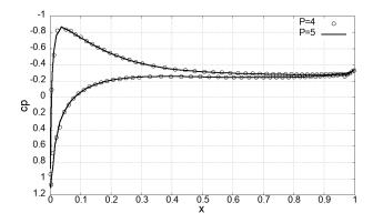
Fig. 4: Time-averaged pressure coefficients over the airfoil obtained with two different polynomial orders: P = 4 (empty dots), P = 5 (solid line).
