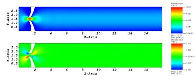
Fig. 2: Full order, steady-state solution for v = 10: velocity in x-direction (top) and y-direction (bottom).
