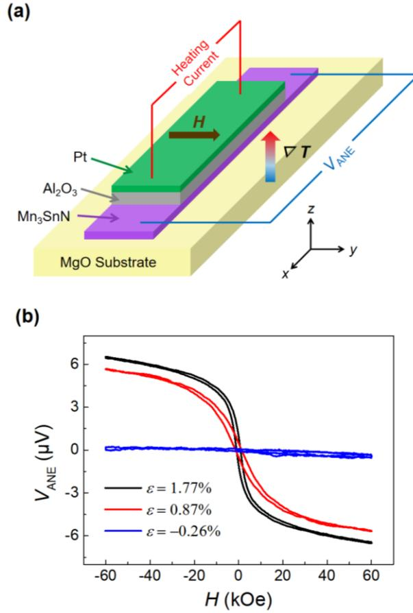
FIG. 3. (a) Schematic of the measurement of anomalous Nernst effect. The temperature gradient  $\nabla T$  is applied out of plane along the  $z$  axis by the Pt heater. The magnetic field is applied in plane along the  $y$  axis. The anomalous Nernst voltage  $V_{ANE}$  is measured along the  $x$  axis. (b) Magnetic field dependence of  $V_{ANE}$  for films with different biaxial strain  $\epsilon$  measured at 100 K. The applied electrical current for heating is 15 mA.
