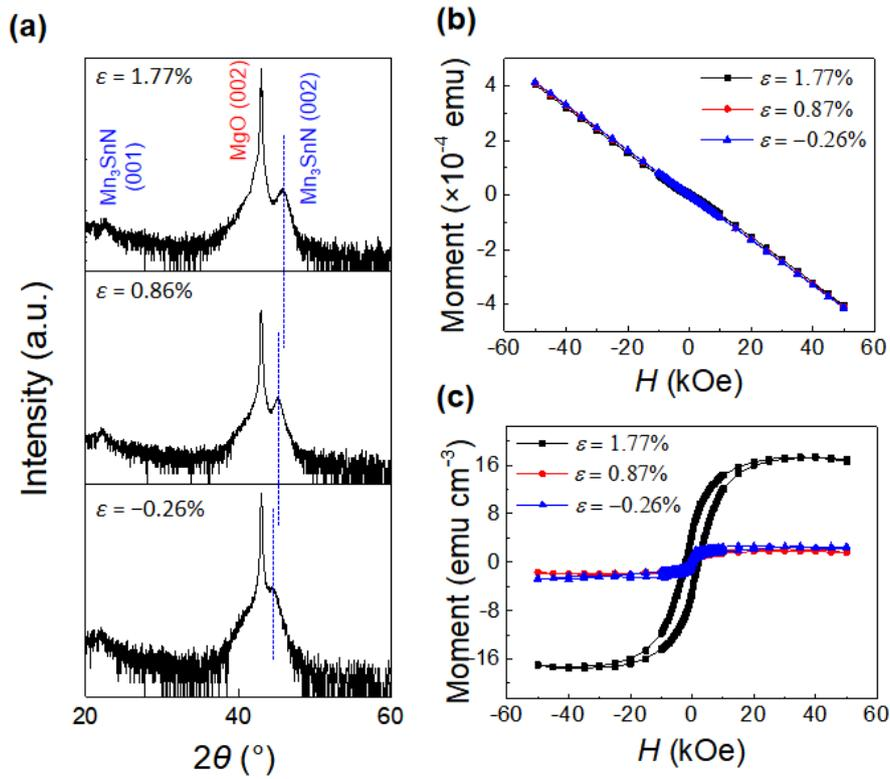
FIG. 2. (a) XRD patterns of the (001)-oriented  $\text{Mn}_3\text{SnN}$  films deposited on  $\text{MgO}$  (001) substrate with different biaxial strain  $\varepsilon$ . Magnetization curves of the  $\text{Mn}_3\text{SnN}$  (001) films with different biaxial strain  $\varepsilon$  by applying an in-plane magnetic field (b) with and (c) without diamagnetic background from the substrate at 100 K.
