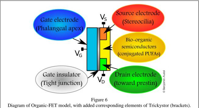
We will consider its elements in turn: the source (Cf. Si 10 A), the semiconductor channel, the gate with its electrical insulation from the overall structure, and, finally, the drain. The source is identical to what has been shown in the classical literature: Electrical potentials result from stereociliae movement (flexoelectricity) and from the biasing potential.
