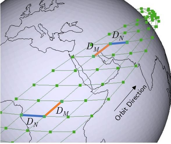
Fig. 3. As satellites within a plane are evenly spaced along their orbit,  $D_M$  remains constant.  $D_N$  is larger near the equator as satellites in adjacent planes are closer near the poles. Adjacent, connected planes all orbit in the same direction.
