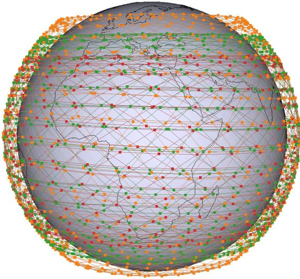
Fig. 1. The proposed Kuiper constellation comprises three shells: 1,156 satellites at 630km/51.9° (orange), 784 at 590km/33° (red), 1,296 at 610km/42° (green) [12].
