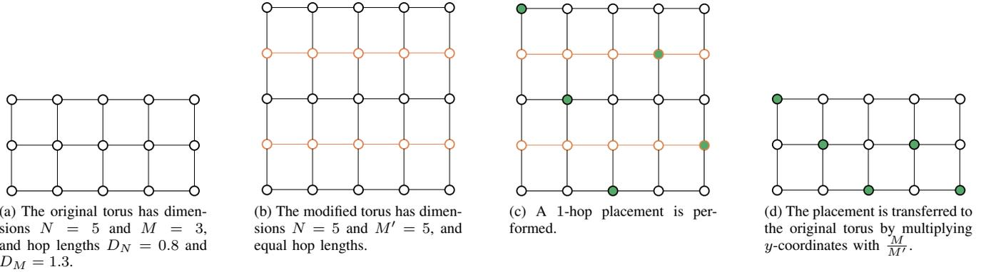
Fig. 4. Placing resource nodes with distance  $d = 1.4$  on a  $5 \times 3$  torus with  $D_N = 0.8$  and  $D_M = 1.3$  (4a, wraparound edges not shown): the torus is extended to  $5 \times \lceil 3 \frac{D_M}{D_N} \rceil$  (4b), then a  $\lfloor \frac{d}{D_N} \rfloor$ -hops placement is performed (4c). Finally,  $y$ -coordinates are transferred by multiplying with  $\frac{3}{5}$ , yielding the resource placement on the original torus (4d).
