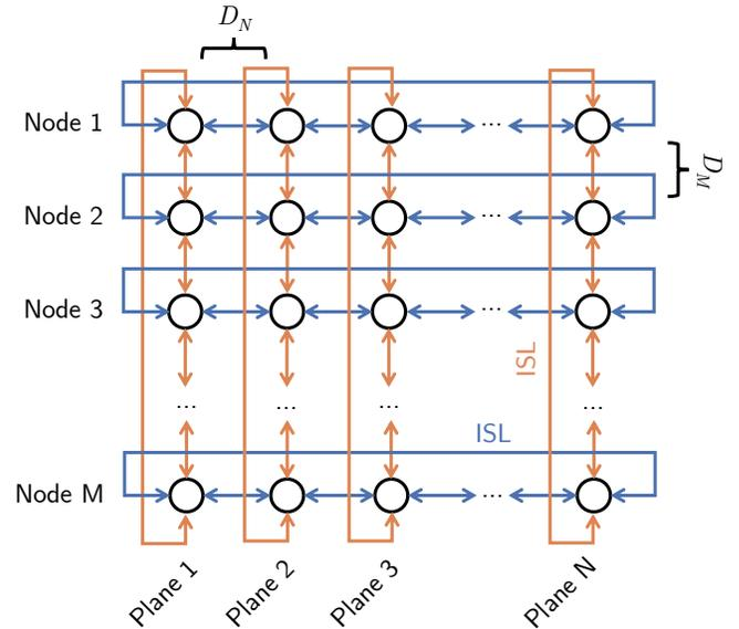
Fig. 2. The satellite network with its ISLs can be modeled as an  $N \times M$  2D torus, where  $N$  is the number of orbital planes and  $M$  is the number of satellites per plane. The length of a hop is constant within an orbital plane but can vary between adjacent nodes over the satellite’s orbital period.
