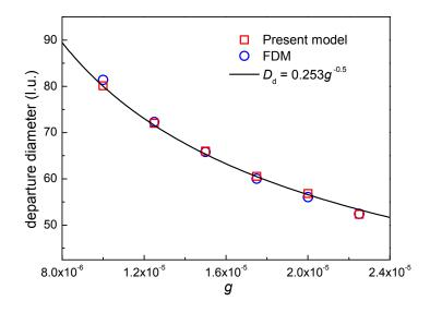
**Fig. 7**. Simulations of bubble nucleation and departure. Numerical validation of the power-law relationship between the bubble departure diameter and the gravitational acceleration.
