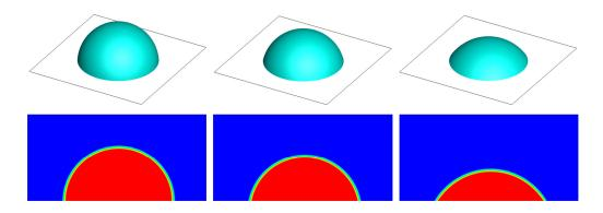
Fig. 5. Snapshots of the density contours obtained by the present model during droplet evaporation on a heated surface. From left to right:  $t = 10000\delta_t$ ,  $90000\delta_t$ , and  $180000\delta_t$ , respectively. A 3D view is shown in the top row with  $x \in [50, 150]$ ,  $y \in [50, 150]$ , and  $z \in [0, 50]$ , while in the bottom row the density contours of the *y-z* cross section at x = 100 are presented.
