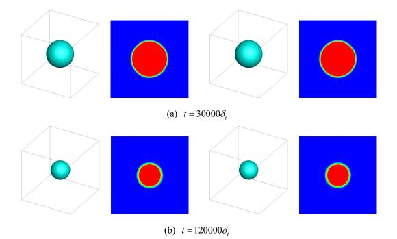
Fig. 2. Numerical validation of  $D^2$  law. Snapshots of the density contours obtained by the present thermal LB model (left) and a hybrid thermal LB model with a finite-difference algorithm (right).
