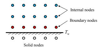
**Fig. 1**. Two-dimensional sketch of the grid nodes near a solid wall. The blue nodes are internal fluid nodes, the red nodes are boundary nodes, while the nodes beneath the solid wall are solid nodes.
