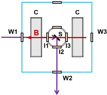
FIG. 1. Principle drawing of the THz-EPR-E setup. A split-coil (C,C) superconducting magnet produces field  $B$  with direction along the incident beam. External (W1, W2, W3; polymer) and internal (I1, I2, I3; diamond) windows separate coils and sample (S) inside the cryostat. A polarization state generator and polarization state detector (not shown) create and analyze state of polarization before and after the sample, respectively.
