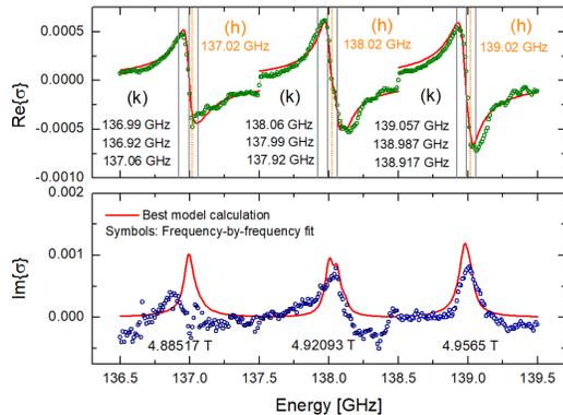
FIG. 5. Symbols: Real (top) and imaginary (bottom) frequency-by-frequency best-match model calculated magnetic function  $\sigma$  defined in Eq. 2. Solid lines: Best-match model calculated lineshape functions defined in Eq. 3. Vertical lines indicate frequencies listed for the  $k$  and  $h$  site triplets at the given magnetic field values, obtained from the lineshape functions and literature data as described in Table I.
