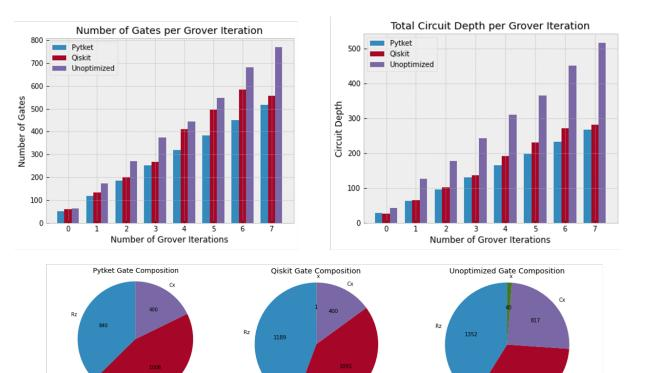
FIG. 5: Depth, gate count, and gate composition of various compilation methods
