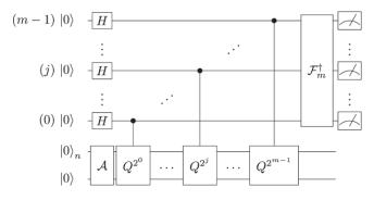
FIG. 1: Canonical algorithm for Amplitude Estimation by Quantum Phase Estimation.
