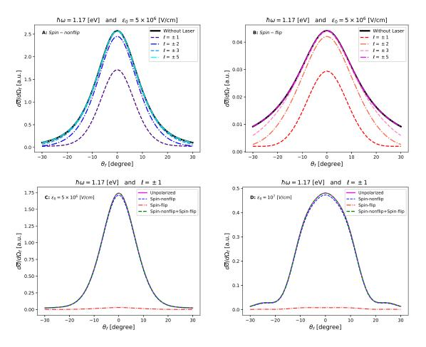
Figure 3: Variation of the summed laser-assisted DCS (38) for polarized electrons as a function of the scattering angle  $\theta_f$  for different summations over  $\ell$ . The notation  $\ell = \pm i$  means that we have summed over  $-i \leq \ell \leq +i$ .
