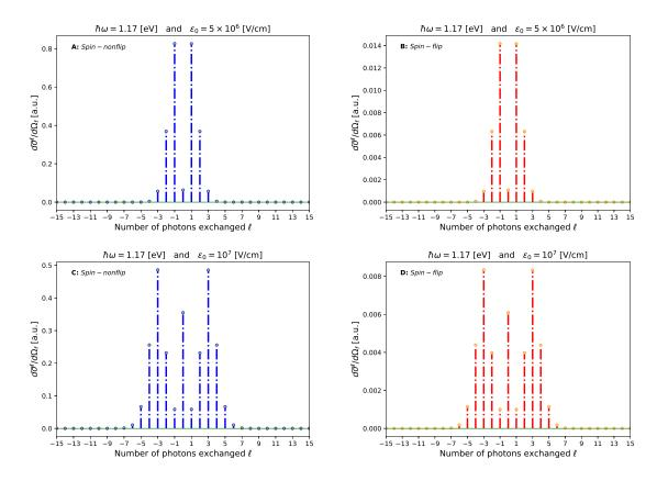
Figure 2: Differential cross section  $d\overline{\sigma}^{\ell}/d\Omega_f(\lambda_1,\lambda_3)$  for spin-flip  $(\lambda_1 = -\lambda_3 = 1)$  and spin non-flip  $(\lambda_1 = \lambda_3 = 1)$  as a function of the number of photons exchanged  $\ell$ . The scattering final angle is  $\theta_f = 0^\circ$ . The field strength  $\varepsilon_0$  and frequency  $\hbar\omega$  are indicated above each figure.
