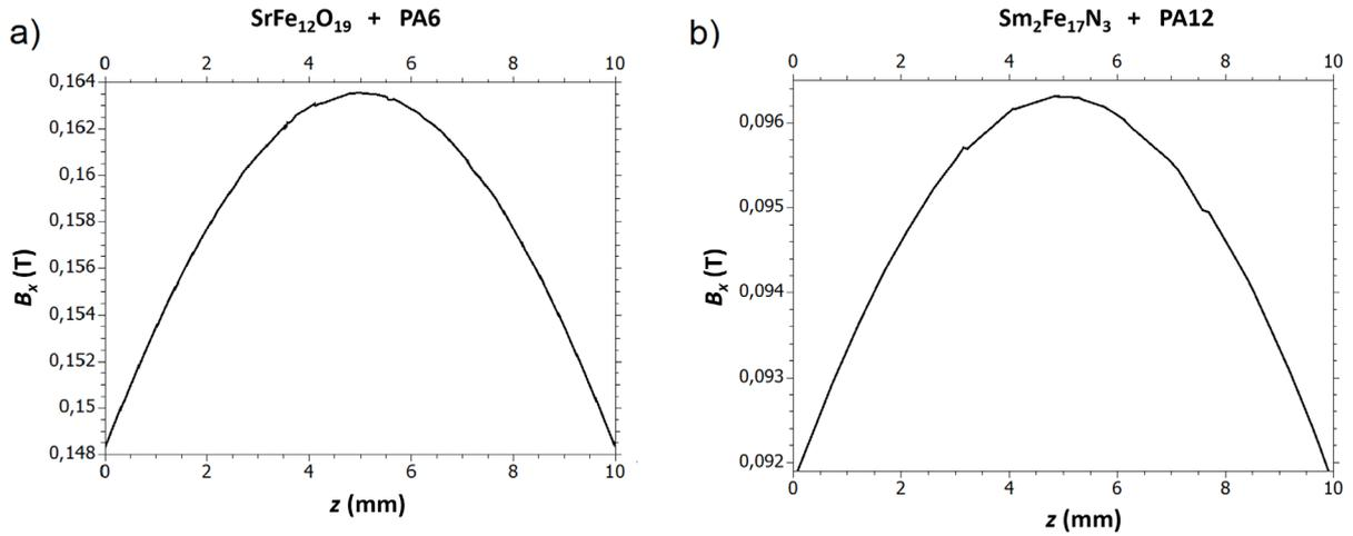
Figure 3: Magnetic flux density  $B_x$  for the hard magnetic distance of a) 15 mm which is suitable for Sprox 10/20p; b) 21 mm which is suitable for  $Sm_2Fe_{17}N_3$ . The zero of  $z=0$  is the end of the nozzle which is equal to the position of the building platform
