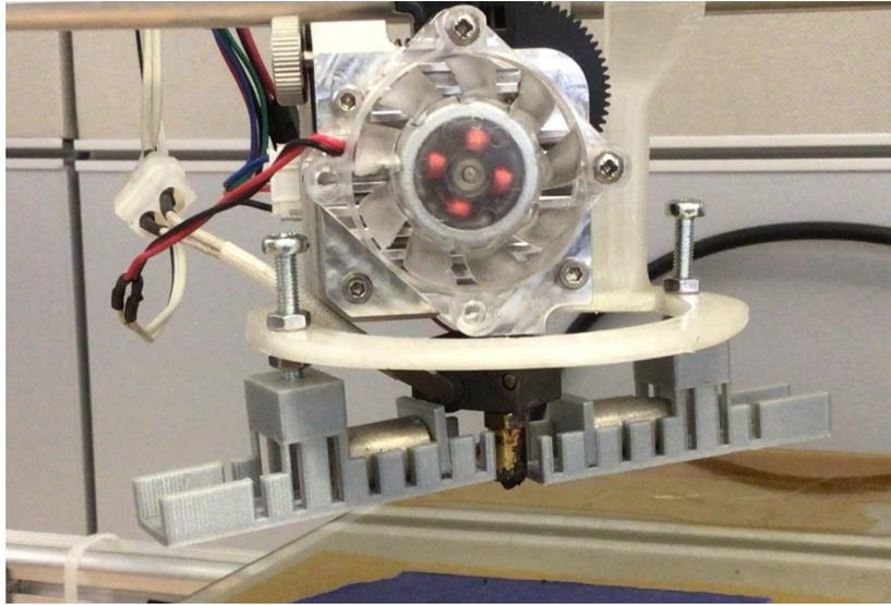
Figure 2: Modified 3D-Printer showing the extruder including the nozzle and the flexible fixing unit for the permanent magnets
