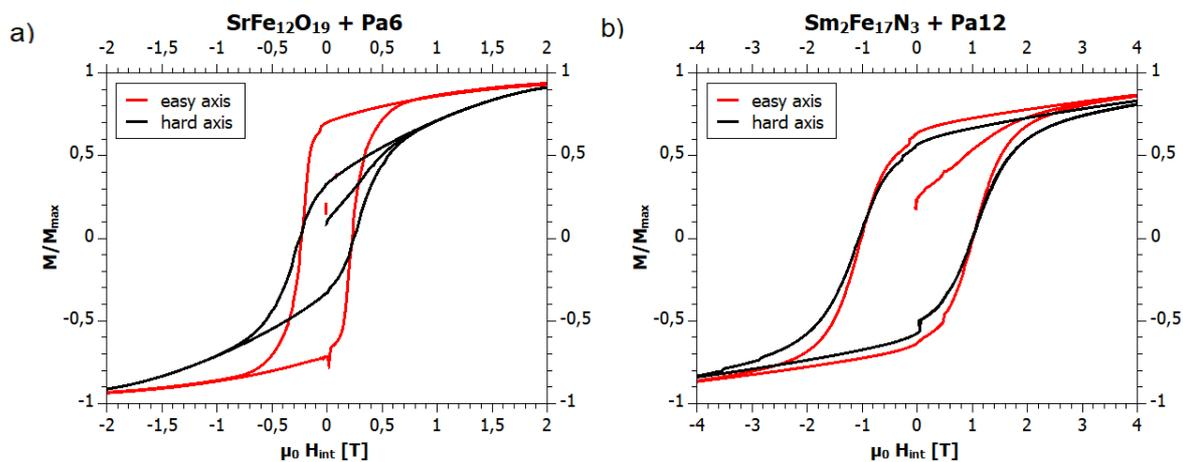
Figure 4: Hard axis and easy axis hysteresis loops of the (a)  $\text{SrFe}_{12}\text{O}_{19}$  (Strontium hexaferrite) and (b)  $\text{Sm}_2\text{Fe}_{17}\text{N}_3$ . Here the easy axis loop denotes the direction that is parallel to the applied field during the printing process.
