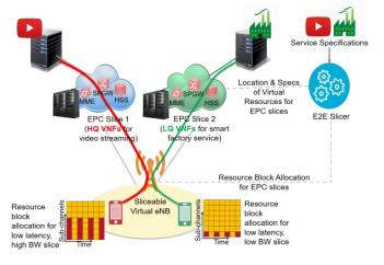
Fig. 2: 5G vertical use cases over the envisioned network slicing architecture.
