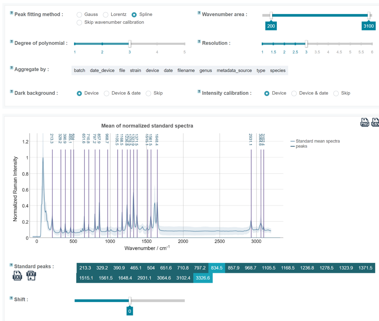
Figure 5 Calibration parameter block. The average measured standard spectrum (here 4-acetamidophenol) is plotted along with the tabled positions of the reference peaks. If different calibration standards should be used, a list of tabled peaks should be imported as a TXT file. The peaks can be added/removed with the buttons below the plot. In case the data has a systematic shift in calibration, it can be specified manually to initially minimize the shift between the tabled and the detected peaks.
