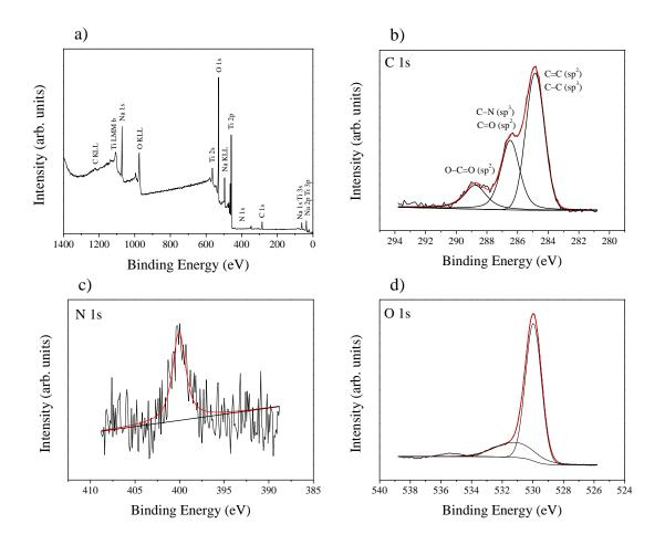
**Figure 7.** a) XPS survey of the C-dots(12.4%)/TNT sample. Graphics b), c) and d) show the high resolution XPS spectra of the C 1s, N 1s and O 1s regions of the same sample, respectively.
