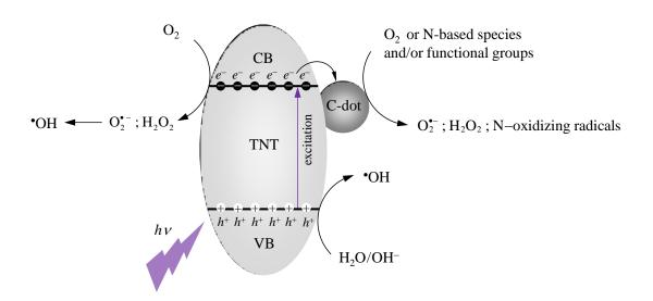
**Figure 10** – Schematic representation of the possible reactive pathways underpinning the photocatalytic activity of the hybrid C-dots/TNT nanomaterials.
