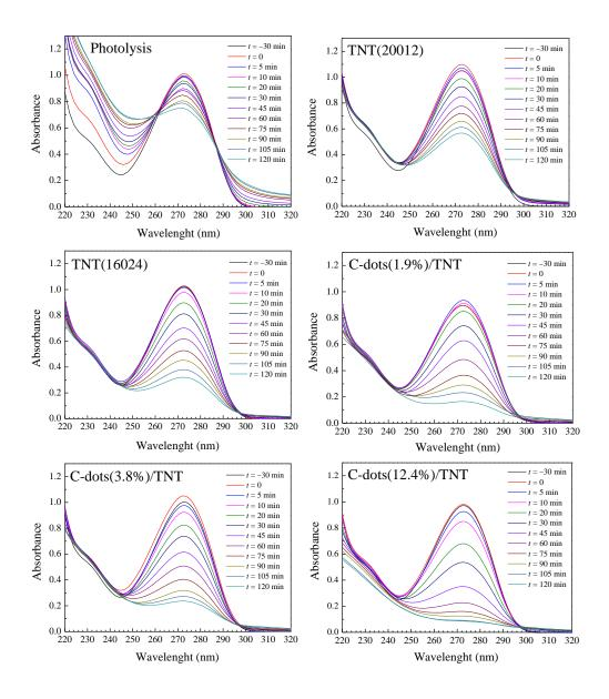
**Figure S5** – Absorption spectra of a 20 ppm caffeine aqueous solutions (150 mL) during photoassisted degradation *via* photolysis and using 20 mg of the prepared samples as photocatalysts.
