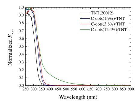
Figure 4 –Normalized absorption spectra of the synthesized samples.
