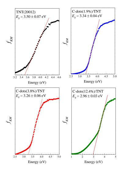
**Figure S4** – Tauc plots obtained for samples TNT(20012), C-dots(3.8%)/TNT, C-dots(12.4%)/TNT and C-dots(12.4%)/TNT.
