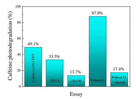
**Figure 9** – Photocatalytic degradation of aqueous caffeine solutions (150 mL, 20 ppm) using 20 mg TNT/C-dots(12.4%) in the absence/presence of scavengers and  $O_2$ , for an irradiation time of 30 min.
