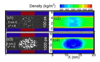
Figure 5: Evolution of vapor bubble using molecular visualization and density contours at initial bubble growing phase (0.1 ns) and final steady-state (1.0 ns) for 5 nm-height nanochannel for  $\varepsilon^* = 6$  (Hydrophilic surface).
