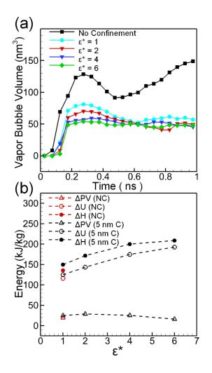
Figure 6: Bubble growth and energy characteristics of bubble nucleation in nanochannel showing (a) vapor bubble volume variation with time, and (b) change in enthalpy, internal energy and work required for bubble nucleation with confinement and hydrophilicity of the surface.
