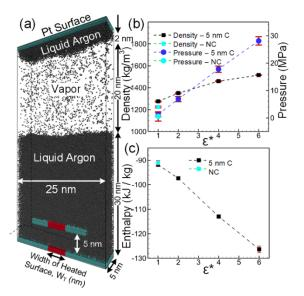
Figure 3: Equilibrium simulations with 5 nm-height nanochannel showing (a) simulation domain, (b) density and pressure variation with  $\epsilon^*$ , and (c) absolute enthalpy of liquid argon variation with  $\epsilon^*$ .
