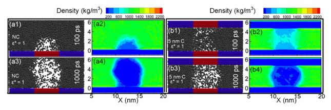
Figure 4: Evolution of vapor bubble using molecular visualization and density contours at initial bubble growing phase (0.1 ns) and final steady-state (1.0 ns) for (a) Not confined liquid with no-channel for  $\varepsilon^* = 1$ , and (b) 5 nm-height nanochannel for  $\varepsilon^* = 1$ ,
