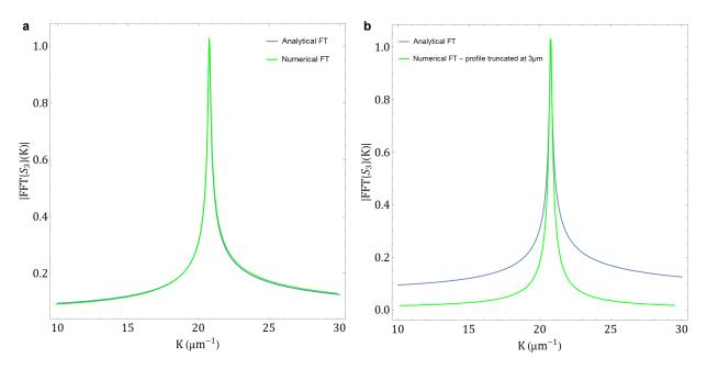
Figure S6: Comparison between the analytical and discrete Fourier transform, (a) for a circular wave profile starting at  $0 \ \mu m$  and (b) for a profile starting at  $3 \ \mu m$ .
