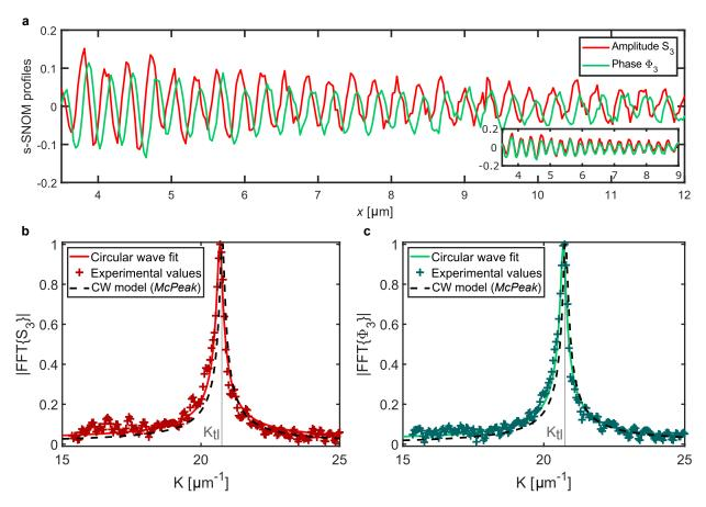
Figure 3: Amplitude and phase at grazing azimutal angle. (a) Comparison of the amplitude and phase profiles at grazing angle. The inset shows the same profiles with the near-field phase shifted by  $-\pi/2$ . (b) Fit of the tip-launched SPPs' amplitude peak visible in Fig. 2(b). The CW model curve refers to the FFT of a circular wave (here Equation 3) where the refractive index from McPeak *et al.*<sup>35</sup> has been used. (c) Fit of the corresponding phase data.
