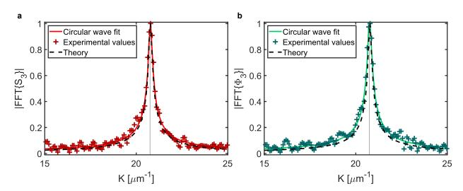
Figure S7: Fit of amplitude and phase at grazing angle ( $\varphi = -1.4^{\circ}$ ), for a starting value  $x_b = 3 \text{ µm.}$  (a) Fit of the tip-launched SPPs' amplitude peak. (b) Fit of the corresponding phase data.
