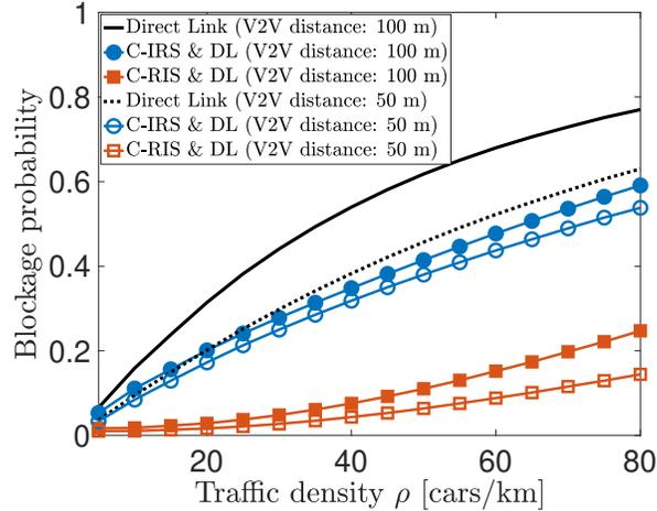
Fig. 10: Blockage probability varying the traffic density
