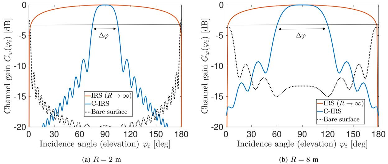
Fig. 5: Channel gain on the elevation plane for a C-IRS compared to a flat IRS ( $R \rightarrow \infty$ ) and a bare cylindrical surface (i.e., without phase compensation) for (5a)  $R = 2$  m and (5b)  $R = 8$  m.
