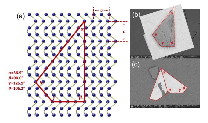
Figure S12. Origin of the etch pits in 2D Te. (a) The shape of etch pits (red dash lines) engraved on right-handed Te  $(10\overline{1}0)$  facet. The etch pits are opposite in a left-handed tellurium flake. (b) Typical etch pits for a right-handed Te. (c) 2D Te flakes after sulfuric etching showing outline shapes similar to etching pits.
