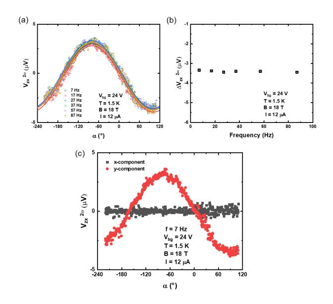
**Figure S6. Frequency-dependent nonlinear planar Hall effect.** (a) Angular-dependent nonlinear planar Hall signal  $(V_{zx}^{2\omega})$  at different lock-in frequencies. (b) The amplitude of nonlinear planar Hall effect  $\Delta V_{zx}^{2\omega}$  extracted from (a). The signals show no significant frequency dependence. (c) The x-component and y-component of the second-harmonic transverse voltage drop  $V_{zx}^{2\omega}$  measured by lock-in at the frequency of 7 Hz.
