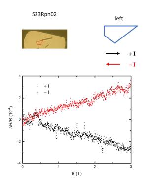
Figure S13. Additional nonreciprocal electrical transport data on left-handed 2D Te.
