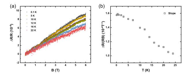
Figure S3. Temperature dependence of the nonreciprocal electrical transport. (a) Temperature dependence of the nonreciprocal electrical transport in a p-type 2D Te FET. (b) Temperature dependence of  $\frac{\Delta R}{RB}$  extracted using the linear fitting of the data from (a).
