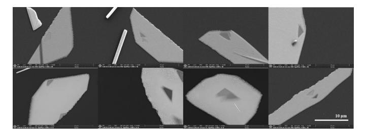
Figure S11. SEM pictures of the etch pits in right-handed 2D Te single crystals.
