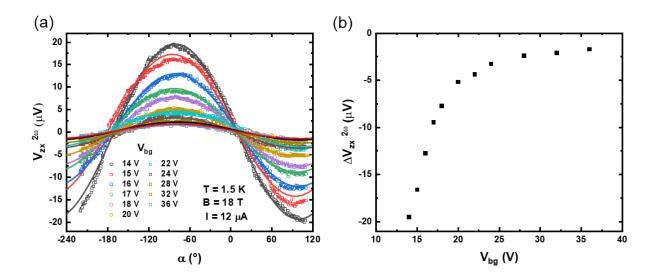
Figure S8. Back gate voltage dependence of the nonlinear planar Hall effect. (a) The second harmonic transverse voltage  $V_{zx}^{2\omega}$  as a function of the magnetic field angle  $\alpha$  at different back gate voltages  $(V_{bg})$ . The solid lines are curves fitting by  $\Delta V_{zx}^{2\omega} \sin(\alpha)$ . (b) Back gate voltage  $V_{bg}$  dependence of the second harmonic transverse voltage amplitude  $\Delta V_{zx}^{2\omega}$  extracted from (a).
