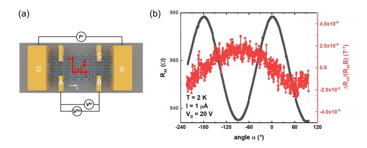
**Figure S4. Angular-dependent longitudinal nonreciprocal transport with an in-plane magnetic field.** (a) Schematic of the in-plane magnetic field measurement setup. (b) Firstorder (black) and second-order (red) angular-dependent magnetoresistance. Small nonreciprocal current is observed when the magnetic field is perpendicular to the current. No nonreciprocal transport is observed when the magnetic field is parallel to the current.
