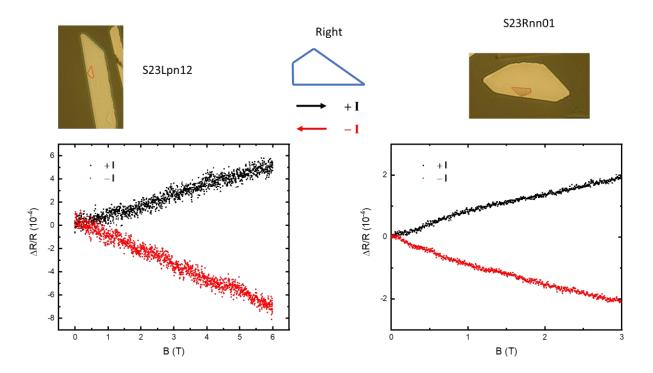
Figure S14. Additional nonreciprocal electrical transport data on right-handed 2D Te.
