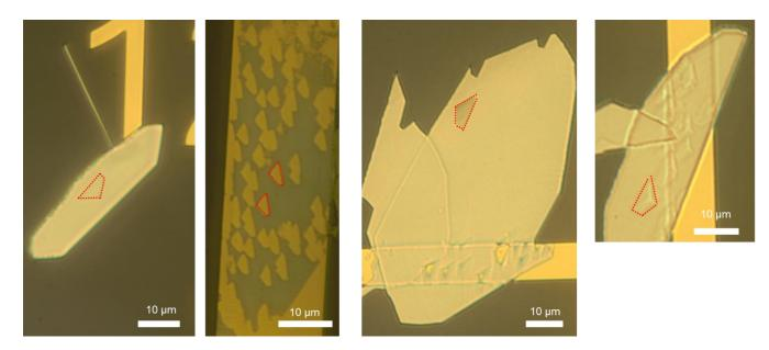
Figure S9. Optical images of the etch pits in 2D Te flakes.
