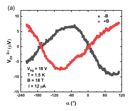
Figure S5. Nonlinear planar Hall effect in positive and negative magnetic field. Nonlinear planar Hall signal  $(V_{zx}^{2\omega})$  with positive and negative magnetic field.
