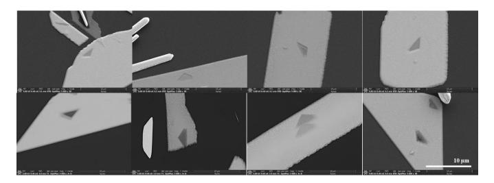
Figure S10. SEM pictures of the etch pits in left-handed 2D Te single crystals.
