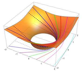
FIG. 1: Regular geodesics embedded on half of the MT wormhole with turning points at  $r_t = 2.0, 1.5, 1.25, 1.125, 1.0625, 1.03125, and 1.01581$ . Here b = 1. The critical  $2\pi$ -encircling geodesic orbit with  $r_{t1} = 1.01581$  is displayed as a dashed line.
