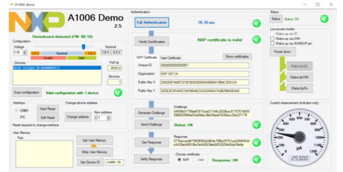
Fig. 18. Graphical user interface for an evaluation of the NXP A1006 secure authenticator. Full Authentication takes about 79 ms.
