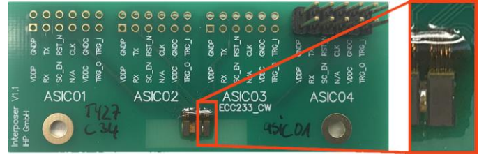
Fig. 3. IHP kP accelerators produced in IHP's 250 nm technology bonded to a PCB and a zoomed in die.
