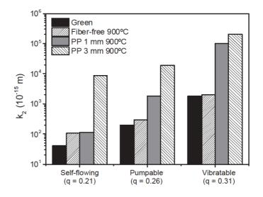
Figure 9: Combined effect of PSD and fiber length on castable's permeability (adapted from [32]). A total of 0.36 vol% of polypropylene fibers (1 mm or 3 mm long and 15 µm diameter) was added to the refractories.
