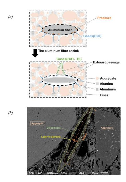
Figure 17: (a) Sketch of the aluminum fiber shrinkage and the formation of permeable paths when the generated gas escape from the resulting structure. (b) SEM image of the closed pore left by aluminum fiber in the  $Al_2O_3$ -SiC-C castable microstructure after firing at 1500°C. Amount of added Al fiber = 0.20 wt.% [78].
