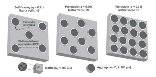
Figure 6: Schematic view of the particle size distribution (PSD) in different classes of refractory castables pointing out the amount of coarse aggregates, the volume content of fine particles (matrix fraction) and permeable interfaces observed in the resulting microstructure [32].
