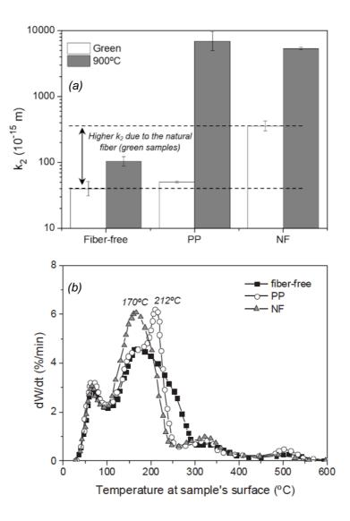
Figure 3: (a) Permeability constant (k<sub>2</sub>) of green and fired samples (900°C) [18] and (b) drying rate for green and humid castables containing polypropylene (PP) or natural fibers (NF). A heating rate of 10°C/min was applied during the thermogravimetric measurements [48]. Dashed lines presented in (a) points out the permeability increase derived from the NF action when compared to the reference composition.
