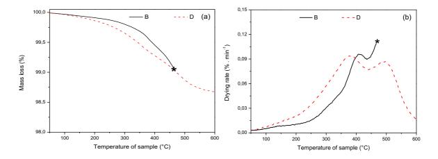
Fig. 23: Mass loss (a) and drying rate (b) of Al<sub>2</sub>O<sub>3</sub>-MgO compositions B (without silica) and D (with 1.0 wt.% of SioxX-Mag) obtained for thermal treatments carried out with heating rate equal to 20°C/min. The analysed samples were previously cured at 50°C/24h and dried at 110°C/24h. The asterisk (\*) indicates the explosion of sample B [92].
