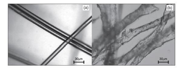
Figure 12: Optical microscopy images of the propylene fibers: (a) as received (smooth, translucent surface) and (b) after mixing step (opaque, scratched surface) of the refractory castables [76].
