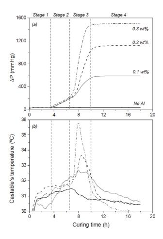
Figure 15: Stages of hydrogen generation as a function of the curing time and aluminum (uncoated metal powder) content incorporated into aluminous refractory compositions. (a) Pressure increase and (b) castable's temperature profiles. The curing process was carried out at 30°C [81].
