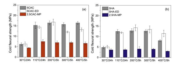
Figure 22: Cold flexural strength evolution of (a) calcium aluminate cement (CAC) or (b) hydratable alumina (HA)-bonded castables obtained after curing  $(30^{\circ}C/24h)$ , drying  $(110^{\circ}C/24h)$  and firing (200-400^{\circ}C/5h). ED = polymeric fibers and MP = permeability enhancing active compound [89].
