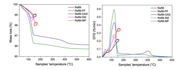
Figure 24: (a) Mass loss (%) and (b) first derivative of the mass loss curve for the thermal treatments carried out with a heating rate of  $20^{\circ}$ C/min for the Al<sub>2</sub>O<sub>3</sub>-MgO castables. All samples were cured at 30°C for 1 day before the measurements. PF = polymeric fibers, OAS = aluminum lactate, SM = silica-based additive and MP = Refpac Mipore 20 (PEAC) [37].
