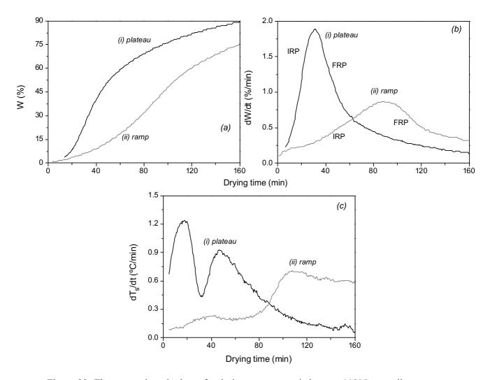
Figure 29: Thermogravimetric data of a drying process carried out at 110°C according to two different heating routines. (a) cumulative water loss (W) and (b) drying rate profiles of the evaluated samples. (c) Heating rate values at the sample's surface. All tests were conducted with a dry air stream inside the furnace. IRP = increasing rate period, FRP: falling rate period [31].
