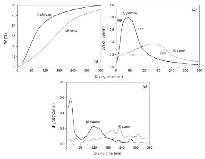
Figure 28: Thermogravimetric data of a drying process carried out at 60°C according to two different heating routines. (a) cumulative water loss (W) and (b) drying rate profiles of the evaluated samples. (c) Heating rate values at the sample's surface. All tests were conducted with a dry air stream inside the furnace. IRP = increasing rate period, FRP: falling rate period [31].
