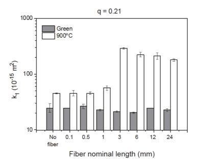
Figure 11: Permeability versus fiber length for self-flowing castables (q = 0.21) [75].
