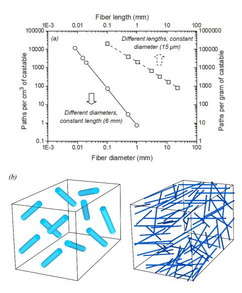
Figure 13: (a) Number of paths formed in the castables' structure after fibers' burnout as a function of the diameter (fixed length = 6 mm) and length (constant diameter = 15  $\mu$ m) of these additives, considering the same added amount (0.36 vol%). (b) Sketch of the thick and thin fiber distribution in the castables' structure (for the same length and volumetric content) [75].
