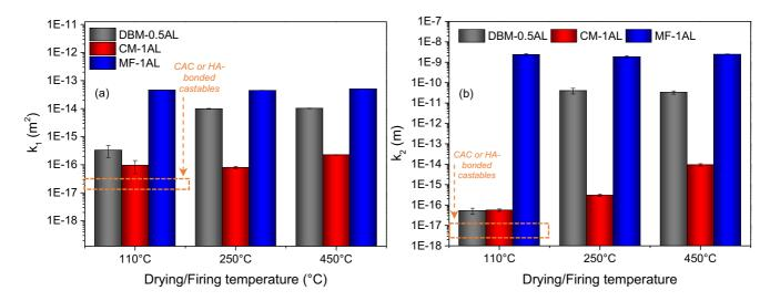
Figure 25: Permeability constants (a)  $k_1$  and (b)  $k_2$  measured for the dried and fired samples of the aluminum lactate-containing castables. DBM = dead burnt magnesia, CM = caustic magnesia and MF = magnesia fumes [110].
