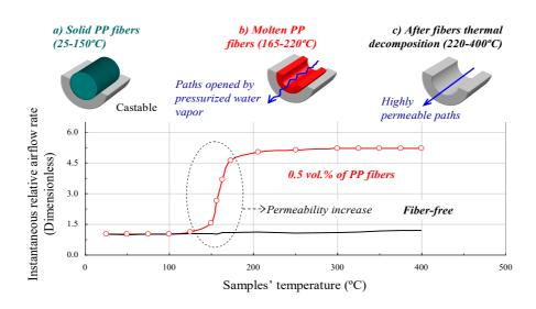
Figure 2: Fluid dynamic behavior of polypropylene (PP) fibers containing refractory castables (hot air permeametry) and schematic representation of fibers' permeability increase mechanism (a-c) [46].
