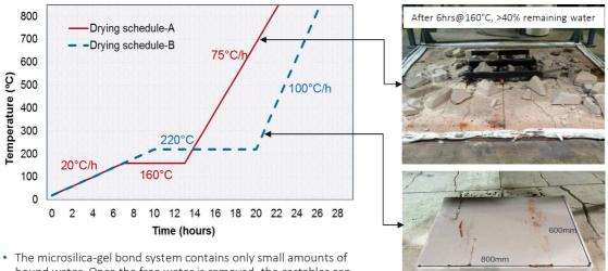
bound water. Once the free water is removed, the castables can be fired at a very high heating rate.
