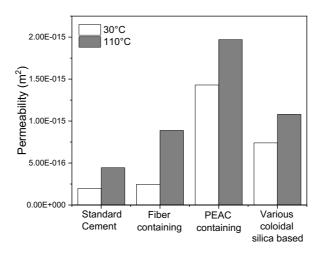
Figure 19: Permeability values ( $k_1$ ) obtained for alumina-based CAC-bonded castables with no drying additive (standard cement), 0.1 wt.% of polypropylene fibers (fiber containing), 2.5 wt.% of a permeability enhancing active compound (PEAC containing). A colloidal silica bonded composition containing 2.5 wt.% of silica fume (various colloidal silica based) was also analyzed [20].
