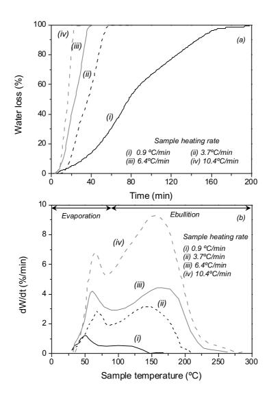
Figure 26: (a) Mass loss profiles as a function of time and (b) drying rate (DTG) of CAC-bonded alumina-based castables. The samples were subjected to distinct heating rates (0.9 to 10.4°C/min) [30].
