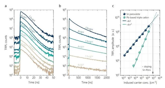
**Figure 4**. **a** and **b**, Injection dependent TRPL transients for a tin-based  $FA_{0.83}Cs_{0.17}Snl_3$  perovskite and a lead-based triple cation perovskite  $Cs_{0.05}(FA_{0.83}MA_{0.17})_{0.95}Pb(I_{0.83}Br_{0.17})_3$ , respectively, as function of the injected carrier concentration. **c**, TRPL amplitude as function of injected carrier concentration corresponding to the same films on **a** and **b**.
