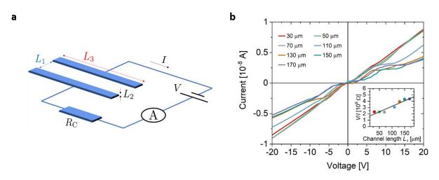
**Figure S5. a**, Scheme of the transfer length method. Here  $L_3=1$  cm and  $L_1$  ranges from 30 µm to 170 µm, **b**, Example of the measurement of the current as a function of the applied bias for different transfer lengths  $L_1$ . In the inset, the quotients V/I are shown for several transfer lengths  $L_1$ . The conductivity is determined from the slope of this line.
