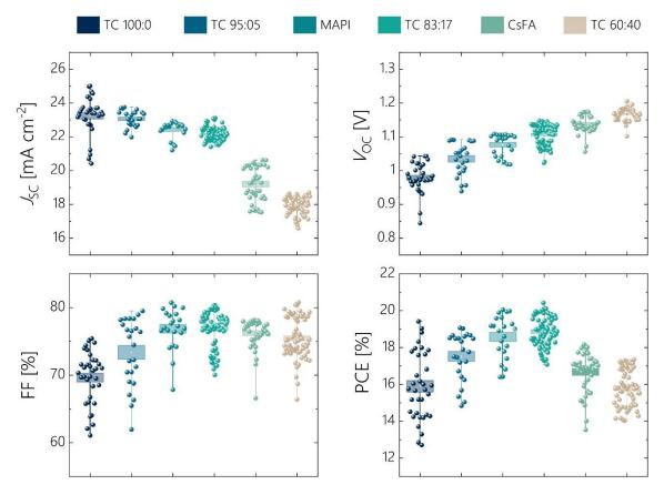
**Figure S3.** Performance parameters of the investigated solar cells. The top labels correspond to the different investigated compositions. Here, "CsFA" refers to  $Cs_{0.15}FA_{0.85}Pb(I_{0.75}Br_{0.25})_3$  and "TC" stands for Triple Cation perovskites  $Cs_{0.05}(FA_xMA_y)_{0.95}Pb(I_xBr_y)_3$  with different percentages of formamidinium lead iodide FAPbI<sub>3</sub> (*x*) and methylammonium lead bromide MAPbBr<sub>3</sub> (*y*), in such a way that x + y = 100%.
