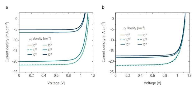
**Figure S6.** Simulated *JV* curves for different doping densities with a mobile cation density of  $10^{17}$  cm<sup>-3</sup>. The simulations were carried out in Fluxim-Setfos. **a**, acceptors  $(p_0)$ . **b**, donors  $(n_0)$ .<sup>64</sup>
