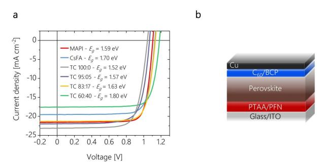
**Figure S2. a**, Current density versus voltage curves of the cells highlighting their bandgap. **b**, Layout of the devices in the inverted *pin*-structure. Here, "CsFA" refers to  $Cs_{0.15}FA_{0.85}Pb(I_{0.75}Br_{0.25})_3$  and "TC" stands for Triple Cation perovskites  $Cs_{0.05}(FA_xMA_y)_{0.95}Pb(I_xBr_y)_3$  with different percentages of formamidinium lead iodide FAPbI<sub>3</sub> (*x*) and methylammonium lead bromide MAPbBr<sub>3</sub> (*y*), in such a way that x + y = 100%.
