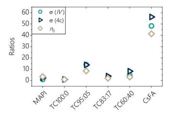
**Figure S4.** Ratios of the independent conductivities and carrier densities to those corresponding to the composition  $Cs_{0.05}FA_{0.95}PbI_3$  which exhibits the lower values.
