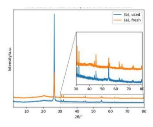
**Figure 2**. XRD patterns of (a) as prepared Sn-gel polymer electrode, and (b) same electrode after 30 charge-discharge cycles.
