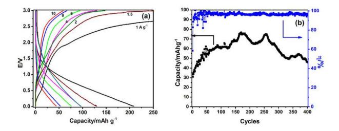
**Figure 4.** (a) Galvanostatic charge-discharge plots at different current densities (indicated) for sodium-ion capacitors prepared using Sn-gel polymer negative electrodes and biomass-based activated carbon positive electrodes with porous polymer film electrolyte, and (b) plots of capacity and Coulombic efficiency with respect to cycles for the same device.
