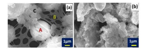
**Figure 1.** Scanning electron micrographs of (a) as prepared Sn-gel polymer electrode (**A**, **B** and **C** denote various regions as explained in text), and (b) same electrode after 30 charge-discharge cycles.
