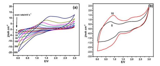
**Figure 3.** (a) Cyclic voltammetry plots at different scan rates (indicated) for sodium-ion capacitors prepared using Sn-gel polymer negative electrodes and biomass-based activated carbon positive electrodes with porous polymer film electrolyte, (b) zoomed CV plots at 5 and 10 mV s<sup>-1</sup> scan rates.
