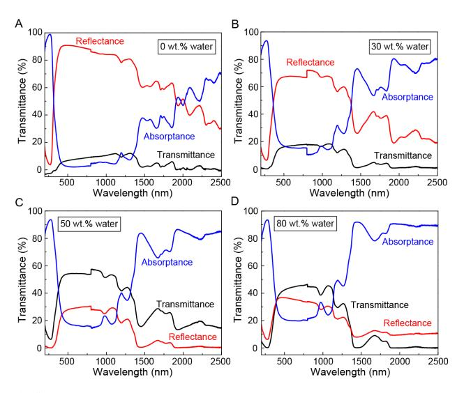
**Fig. S7.** Reflectance, transmittance and absorbance spectra of freeze-dried samples with different water contents: (**A**) 0 wt%, (**B**) 30 wt%, (**C**) 50% wt%, (**D**) 80 wt%. The small discontinuities at 800 nm is due to equipment grating change.
