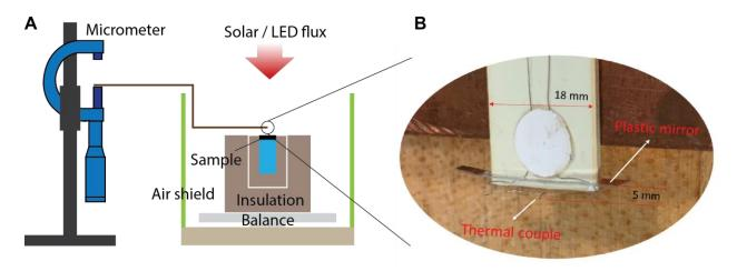
Fig. S12. (A) Illustration and (B) photo of the thermocouple configuration for vapor phase temperature mapping along height direction.
