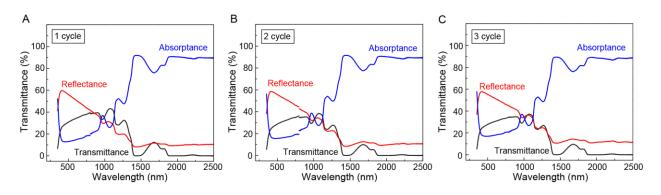
Fig. S6. Reflectance, transmittance and absorbance spectra of freeze-thawed samples (A) 1 freeze-thaw cycle, (B) 2 freeze-thaw cycles, and (C) 3 freeze-thaw cycles.
