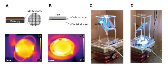
**Fig. S10.** (**A**, **B**) Illustration of PVA-ppy and PVA-carbon electrical heating testing configuration and IR image of surface temperature profile, respectively, (**C**,**D**) photos of a home-made setup that can do solar heating from top and bottom.
