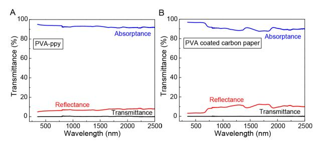
Fig. S9. Reflectance, transmittance and absorbance spectra of (A) PVA-ppy wet sample; and (B) PVA coated carbon paper wet sample.
