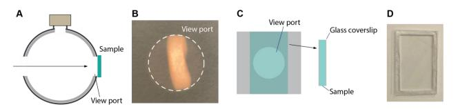
**Fig. S4**. (A) Illustration of sample configuration when using the integrating sphere. (B) Photo of the back port of integrating sphere and probe beam size. (C) Illustration of home-built sample holders for use with integrating sphere, and (D) a photo of the sample holder.
