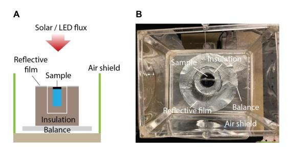
Fig. S8. Illustration (A) and photo (B) of the evaporation rate measurement set up.
