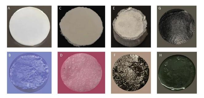
**Fig. S2**. Photos o (**A**) frozen and (**B**) swollen states of freeze-thawed pure PVA sample. (**C**) dry and (**D**) swollen states of freeze-dried pure PVA sample; (**E**) dry and (**F**) swollen states of PVA-PPy sample; (**G**) PPy modified carbon paper at dry state and (**H**) pure PVA coated carbon paper at swollen state.
