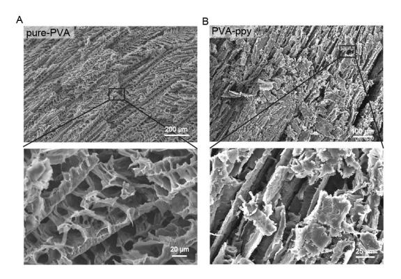
**Fig. S1**. SEM images of (**A**) pure-PVA, and (**B**) PVA-ppy samples. Samples typically show columnar structures running vertically towards surface. The pure-PVA samples have lateral ridges across the vertical columnar structures.
