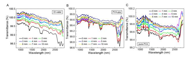
**Fig. S14. Direct transtance spectra of moist air over various samples at different heights**. (A) pure water from 0mm to 10mm; (B) PVA-ppy sample from 0mm to 10mm; (C) Freeze-dried pure PVA sample from 0mm to 10mm. Dry air transmittance, obtained from normalizing the spectra of dry air using an aperture, which limits the spot width in the height direction to ~ 1mm to that without an aperture.
