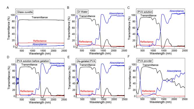
**Fig. S5.** Reflectance, transmittance and absorbance spectra of (**A**) empty glass cuvette; (**B**) DI water; (**C**) PVA solution; (**D**) PVA solution (as-gelated); and (**E**) PVA powder.
