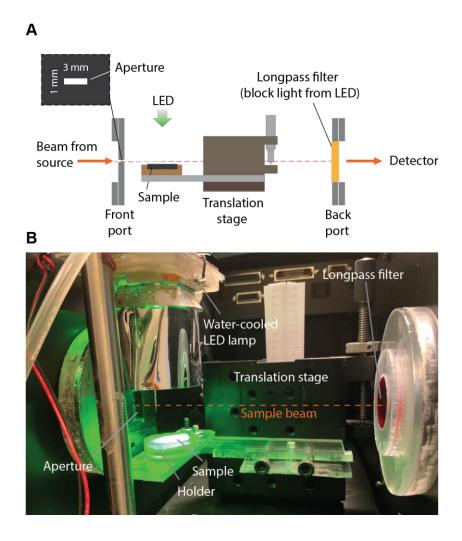
**Fig. S13**. (A) Illustration and (B) photo of a sample stage for vapor phase absorbance measurement inside a Cary 5000 UV-VIS-NIR spectrometer.
