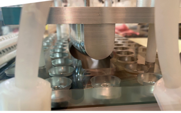
FIG. 10. Side view of the electropolishing setup for the cigar-shaped cavity. The aluminum anode is lowered from above; it was fabricated with geometry to match the cavity.
