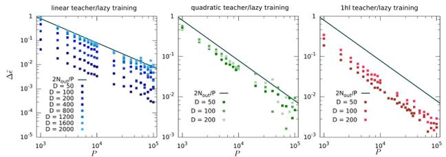
FIG. 6. Generalisation gap of a lazy training architecture as a function of the number of examples in the training set for different input sizes  $D$ . From left to right the teacher functions are respectively linear, quadratic and 1hl. The size of the hidden layer is kept fixed to  $N_{\text{out}} = 400$ .
