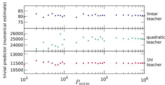
FIG. 5. Numerical estimate of the trivial predictor  $T$  as a function of the number of points  $P_{\text{norm}}$  used in the approximation. These values describe a single realisation of a random teacher function (linear, quadratic, 1hl).  $T$  converges to a fixed value around  $P_{\text{norm}} = 10^6$ , that is the value chosen for all our numerical experiments.
