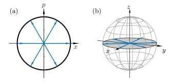
FIG. 1. Sketch of quantum walk on a circle with L = 6 sites. (a) A harmonic oscillator on the phase plane; (b) a spin cluster on the equator of the Bloch sphere. The blue arrows point to the possible locations of the walker.
