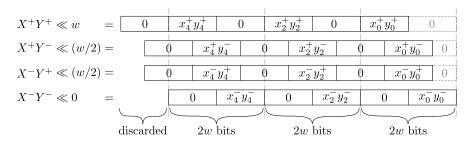
Figure 3: Illustrates step 3 of 2w-bit multiplication. Each of the products  $X^+Y^+$ ,  $X^+Y^-$ ,  $X^-Y^+$  and  $X^-Y^-$  are left-shifted by respectively w, w/2, w/2 and 0 by shifting in zeroes from the right. Then they are added together using componentwise addition for 2w-bit components. Since what we sum up in a 2w-bit component adds up to the product of two w-bit integers, we only need 2w bits to store the result. Hence the addition will not overflow.
