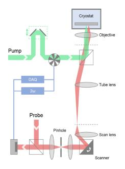
Fig. S1. Schematic illustration of pump-probe confocal optical microscope.
