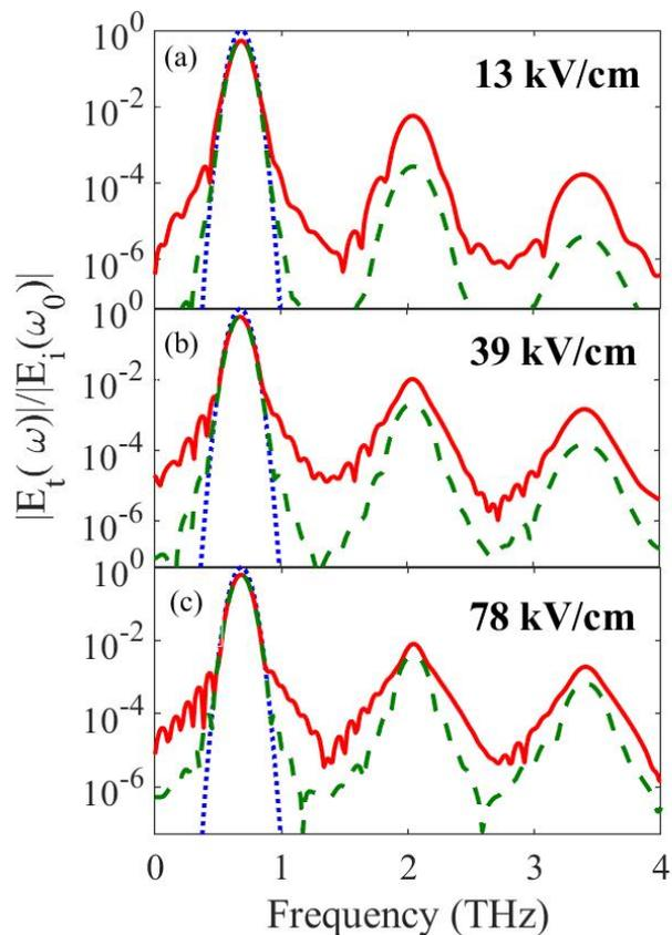
FIG. 9. The Fourier transformed incident field and transmitted field as a function of frequency for input field amplitude of (a) 13 kV/cm, (b) 39 kV/cm, and (c) 78 kV/cm using microscopic model (solid red curve) and semi-empirical model (dashed green curve). The dotted blue curve represents the incident field. The fundamental frequency of the incident field is 0.68 THz and both neutral impurity scattering and optical phonon scattering are included.
