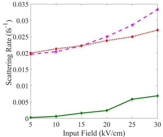
FIG. 5. Extracted effective scattering rate ( $1/\tau$ ) as a function of input field for different scattering treatments; only phonon scattering (solid dark green), impurity scattering (dashed pink curve), and impurity and phonon scattering (dotted red curve).
