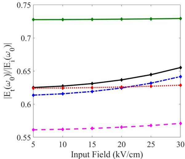
FIG. 4. Ratio of the transmitted field at  $\omega_0$  to the peak value of the incident field as a function of input field as calculated using the simple nonlinear, semiclassical model for scattering times of  $\tau = \infty$  (solid black curve),  $\tau = 4$  ps (dashed-dotted blue curve),  $\tau = 200$  fs (dashed pink curve),  $\tau = 100$  fs (dotted red curve), and  $\tau = 52$  fs (solid green curve).
