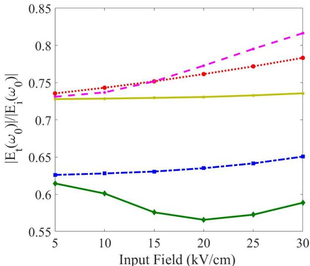
FIG. 2. Ratio of the transmitted field at  $\omega_0$  to the peak value of the incident field as a function of input field for different scattering treatments; only phonon scattering (solid dark green), no scattering (dashed-dotted blue curve), impurity and phonon scattering (dotted red curve), impurity scattering (dashed pink curve), and semi-empirical model (solid light green curve).
