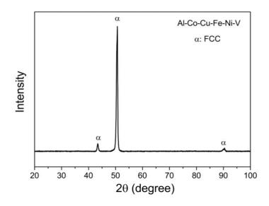
Figure 8. XRD pattern for Al<sub>5</sub>Co<sub>8</sub>Cu<sub>35</sub>Fe<sub>19</sub>Ni<sub>23</sub>V<sub>11</sub>.
