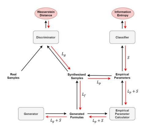
Figure 4. The error backpropagation of generator
