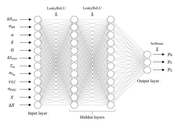
Figure 2. The architecture of the phase classifier in the present study
