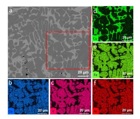
**Figure 9.** (a) BSE SEM image of Al<sub>5</sub>Co<sub>8</sub>Cu<sub>35</sub>Fe<sub>19</sub>Ni<sub>23</sub>V<sub>11</sub>, (b-f) the elemental distribution of Co, V, Cu, Fe and Ni. The area of EDXS mapping is indicated in (a). The map for Al was omitted, as the Al was evenly homogenously distributed throughout the alloy.
