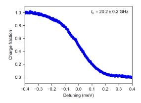
Supplementary Fig. 4. Evaluation of inter-dot tunnel coupling between center and right dot. Charge transition between (1,1,0) and (1,0,1) charge states with the fitting curve<sup>9</sup>. The errors represent the estimated standard errors for the best-fit values.
