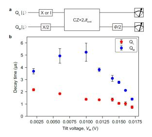
Supplementary Fig. 5. Tilt voltage dependence of  $T_2^*$ , a, Pulse sequence to produce b. The sequence is similar to the one shown in Fig. 3c but the  $\pi$  rotation for both qubits in the middle of the exchange gate is omitted. b, Operation point dependence of  $T_2^*$  which is smaller than that obtained with the decoupled sequence (Fig. 3d). The errors represent the estimated standard errors for the best-fit values.
