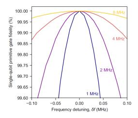
**Supplementary Fig. 9. Simulated frequency detuning dependence of single-qubit gate fidelity.** Simulated single-qubit primitive gate fidelity as a function of frequency detuning (see Supplementary Note 2 for the calculation procedure). Rabi frequency is 1 MHz, 2 MHz, 4 MHz, and 8 MHz for the indigo, purple, orange, and yellow trace, respectively.
