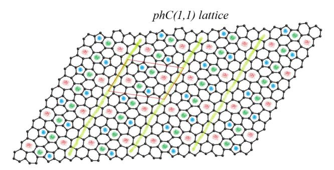
**Figure SI1-10**. a)  $4A \times 4B$  fragment of planar 2D phC(1,1) lattice. Carbon atoms are presented in black. Pentagonal rings are highlighted in blue, heptagonal rings are highlighted in red, and hexagonal rings, which separate pentagonal and heptagonal fragments of the same unit cell, are highlighted in green. Lines of fused hexagons are highlighted in light green. A phC(1,1) unit cell is denoted by rhombus made by red lines.
