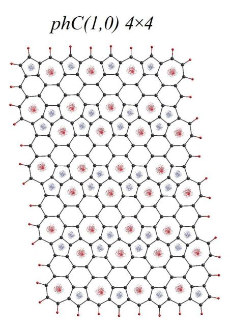
**Figure SI1-7**. A finite fragment (C<sub>232</sub>H<sub>42</sub> flake) of planar  $4 \times 4 phC(1,0)$  lattice. Heptagons are highlighted by red spray and pentagons are highlighted by blue spray. Carbon atoms are presented in black and hydrogen atoms are presented in red.
