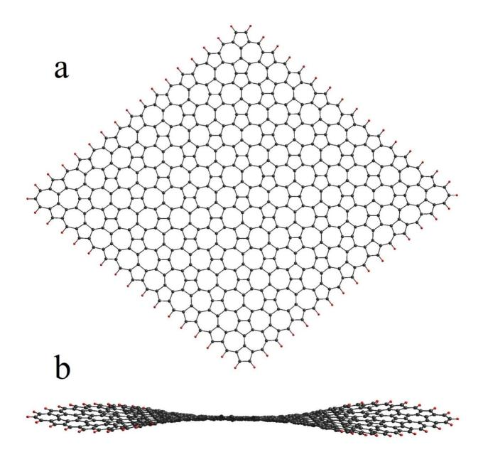
**Figure SI1-3.** Top (a) and side (b) views of PM3  $8 \times 8 \ phC(0,0)$  flake. Bending profile of the flake is clearly seen in the side projection.
