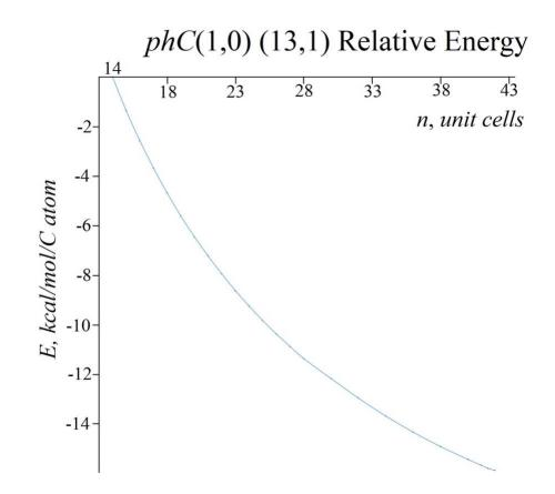
**Figure SI1-9**. The PM3 energy gain (kcal/mol/C atom) of final phC(1,0) (13,1) chiral nanotubes of different lengths with respect to the energy of the shortest completed phC(1,0) (13,1) nanotube constituted by 14 unit cells.
