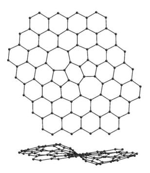
**Figure SI1-2.** Top and side views of carbon backbone of curved conformer of C<sub>96</sub>H<sub>24</sub> cluster (ground state of C<sub>i</sub> or C<sub>s</sub> symmetry) which represents a phagraphene structural unit with double (5/7) core embedded into graphene lattice. The atomic structure was relaxed using both model potential and semiempirical PM3 optimizations.
