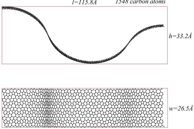
The structure wave box dimensions for  $nA \times 4B$  phagraphene nanoribbons  $l=115.8\text{\AA}$  1548 carbon atoms
