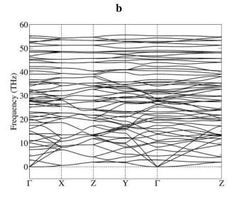
**Figure SI1-6a**. Phagraphene phonon dispersion [1] for 2×2 and 3×3 supercells calculated using PHONON code [3-5]. No imaginary frequencies were detected.
