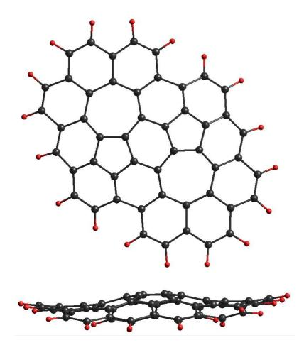
**Figure SI1-1.** Top and side views of minimized curved conformer of C<sub>50</sub>H<sub>15</sub> cluster, which represents two 5/7 phagraphene cores embedded into C<sub>6</sub> environment. Optimization was performed at PM3 and B3LYP/6-31G\* levels of theory with relative energies of planar transition state equal to 5.641 and 0.504 kcal/mol, respectively.
