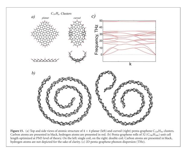
approximately as twice as large as vdW binding energy, one could speculate that after achievement of certain radius at which the resulting curvature of external penta-graphene roll would be rather close to planar structure, strong bending stress should form secondary roll structure with structural passivation of the growing edge, preventing formation of large-diameter penta-graphene rolls.
