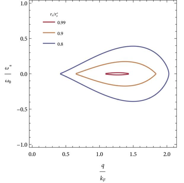
FIG. 6. The imaginary part of the frequency of a new solution of the dispersion equation due to PSOI as a function of wave vector for three values of  $r_s$ . Here a 2D layer in vacuum is considered, its thickness being  $d = 0.02a_B$ , the in-plane dielectric constant  $\epsilon_{\parallel} = 15$ . The PSOI magnitude is  $\tilde{\alpha} = 0.1$ , which corresponds to  $r_s^* = 1.054$ .
